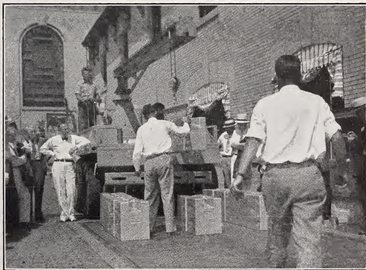
FIGURE 2.—1,000-lb weights being unloaded during test of right end of scale.
