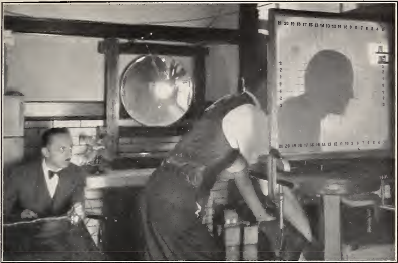
FIGURE 2.— Method of recording positions of observers with respect to scale. The shadow of the observer on the ground-glass screen was photographed. The position of the shadow with respect to the lines on the screen defined the position of the observer with respect to the scale.
