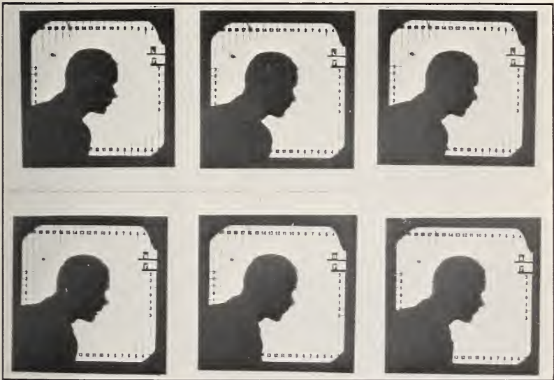
FIGURE 3.— Photographs of an observer having average vision. In the three upper views the observer was viewing the chart direct; in the three lower views he was viewing the chart through the scale lens. The average distance of this observer's eyes from the scale was the same both with and without the lens in place.
