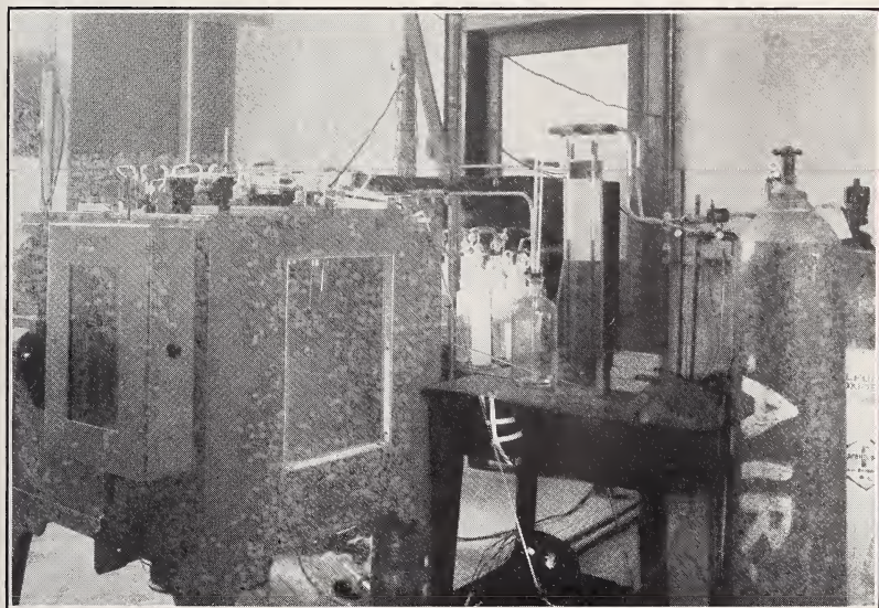
FIGURE 2.— Rear view of apparatus for exposure of paper to sulphur dioxide, showing control accessories.
