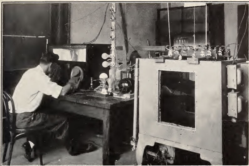
FIGURE 1.— Front view of apparatus for exposure of paper to polluted air showing means of manipulating samples.
