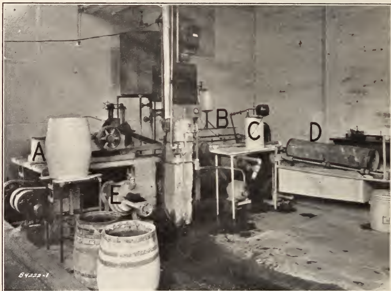
FIGURE 2.— Pulping and screening equipment. A, Beater; B, screen; C, purifier; D, concentrator; E, jordan.
