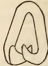
FIGURE 116.—Repair or end lap links
