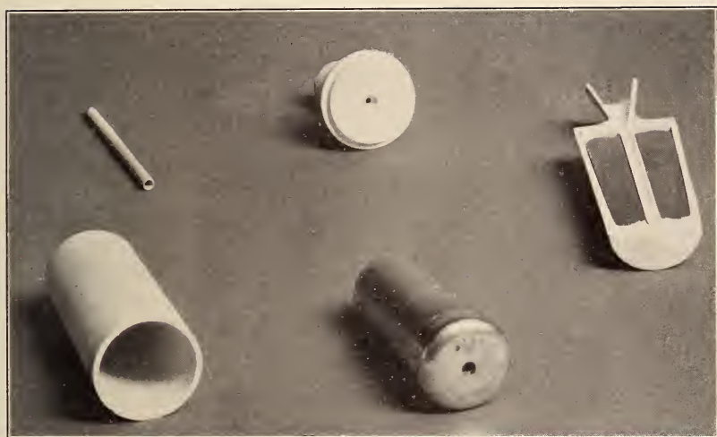
FIGURE 4.— Platinum ingot and parts of crucible used in the black-body standard of light
