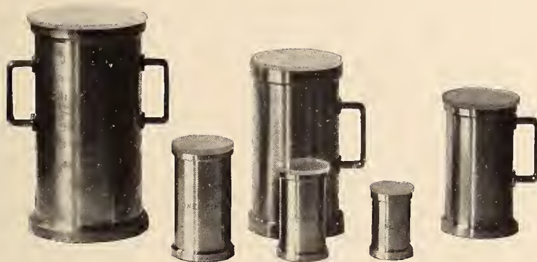
Fig. 2.—Set of liquid capacity measures of simple design and construction suitable as State standards or as primary standards for large cities or manufacturers.
