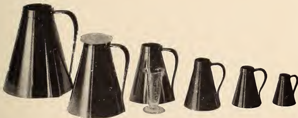
Fig. 3.—Set of conical liquid capacity measures suitable as secondary standards and especially adapted to inspection work.
