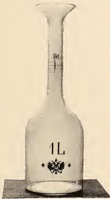
Fig. 4.—Type of glass bottle specially adapted to testing measures. A line on the neck of the bottle defines the capacity and lines above and below the defining line give the tolerances allowed for new and old measures.
