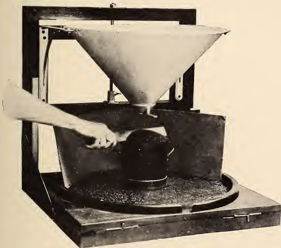
Fig. 5.—Hopper for use in testing measures with seeds, showing the proper method of striking off the surplus seeds from the top of the measure.
