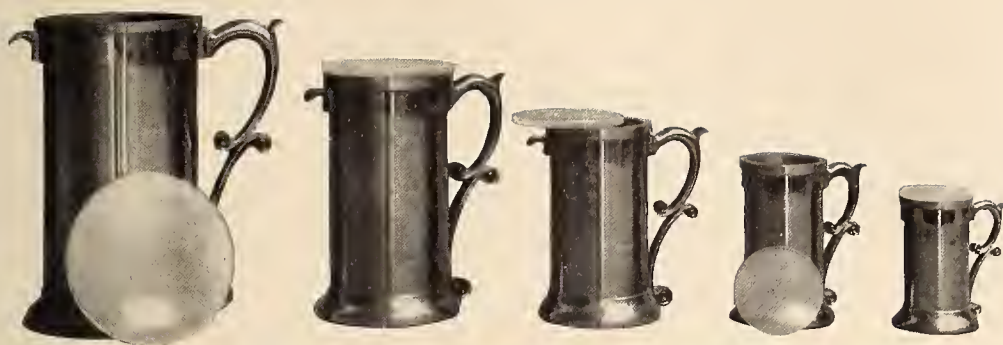
Fig. 1.—Set of liquid capacity measures of heavy construction of the type furnished the States by the National Government as standards 70 years ago.
