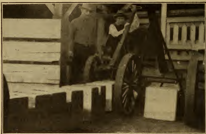
FIGURE 2.—Two-wheeled carts used for shifting 1,000-pound weights during the testing of scales at the Detroit stockyards
