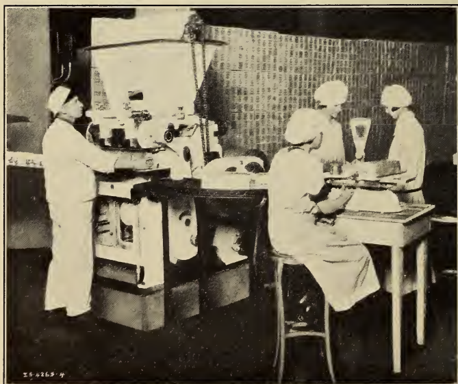
FIGURE 8.—Equipment for filling and check weighing cartons of cheese
