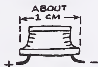
METAL CAPSULE CONTAINING QUARTZ CRYSTAL USED IN WRIST WATCHES
