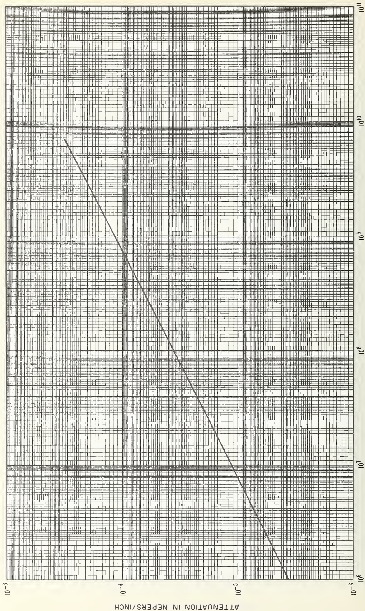
FIGURE 43. Attenuation per inch as a function of frequency under standard conditions for line size #3.
