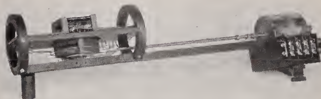
FIGURE 8. Test coil assembly for MH permeameter.
