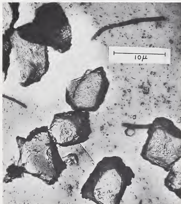
FIGURE 4. Cement paste hydrated 5 min.
