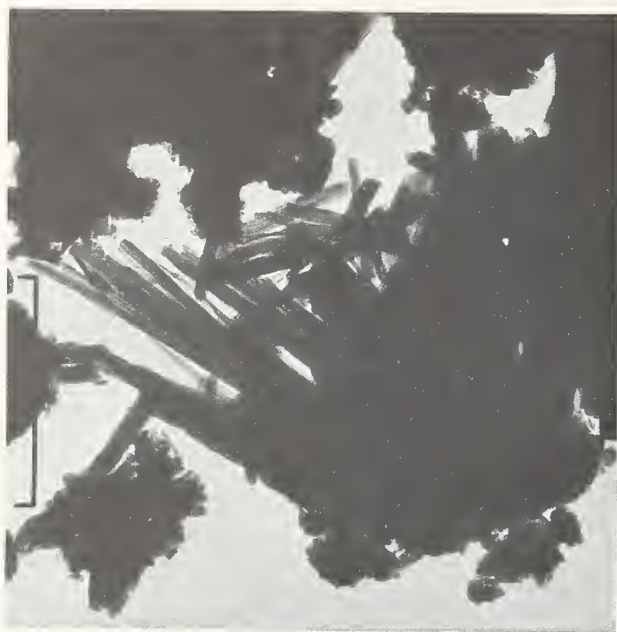
FIGURE 11. Fibrous tobermorite formed in a fully hardened paste of C_3S .
