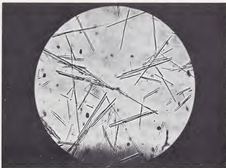
FIGURE 11. Photomicrograph showing crystals of calcium-aluminum hydroxy p -nitro-benzoate.
