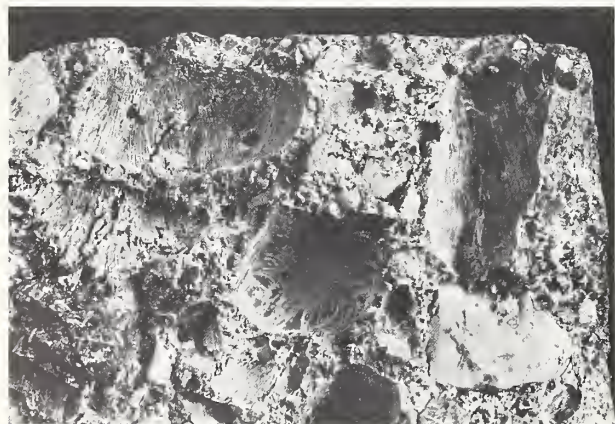
FIGURE 13. Traces of ice needles in concrete frozen after 4 hr prehardening at +20 °C. (Curve 4, fig. 12)
