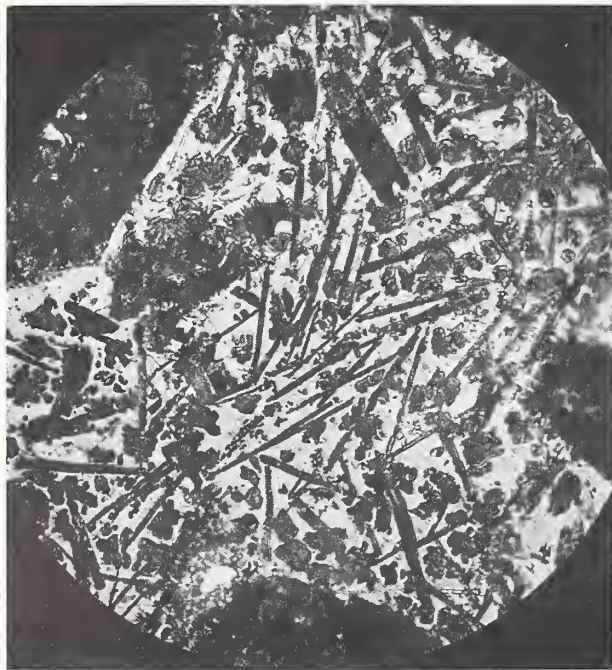
FIGURE 2. Microstructure of granulated clinker. Reflected light. Magnification \times 440 .
