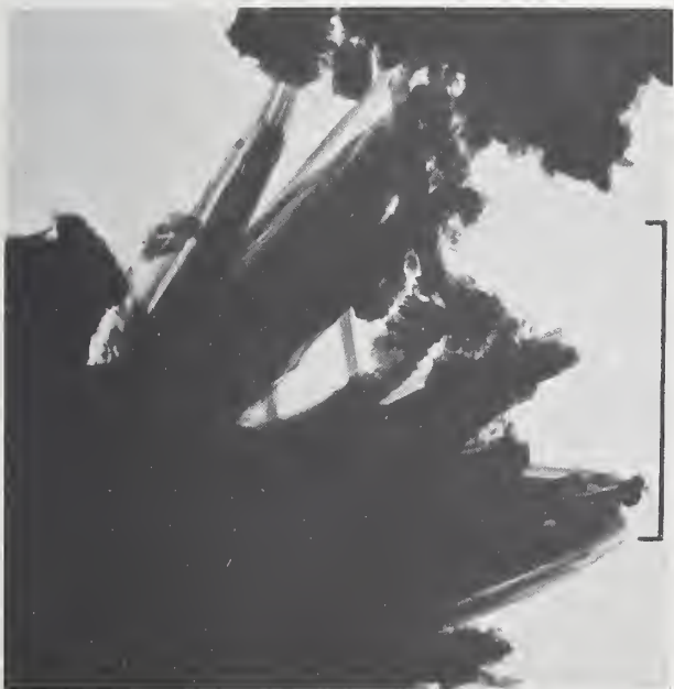
FIGURE 16. Relatively rare fibers from lightly ground hydrated Type I cement paste. w/c=0.55; age=5 months.
