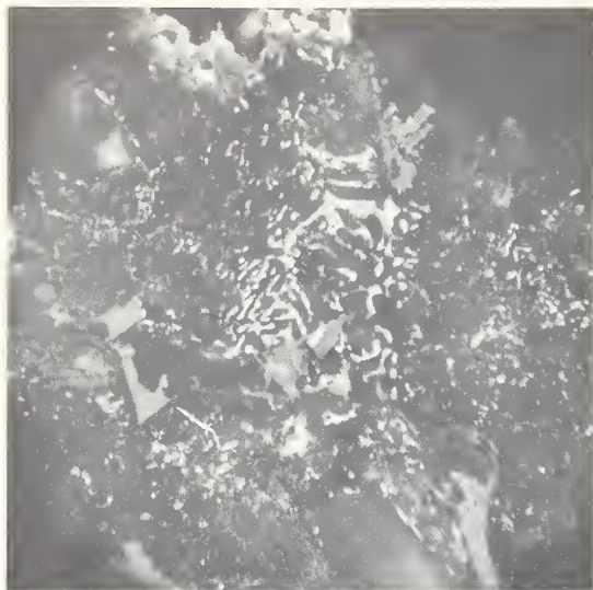
FIGURE 20. Myrmekitic intergrowths of belite, free lime, ferrite, and iron sulfide pseudomorphous after alite. Oil, immersion, crossed nicols. 500 \times .
