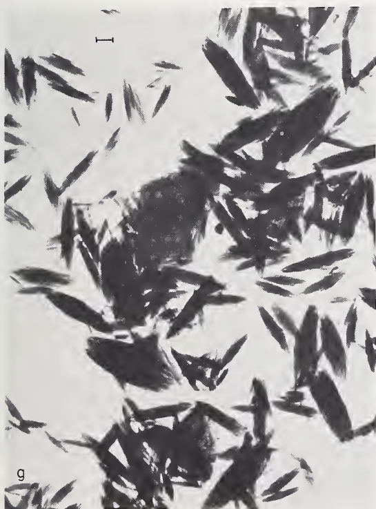
FIGURE 2g. Electron micrograph of hydration products of bottle-hydrated C_2S .
