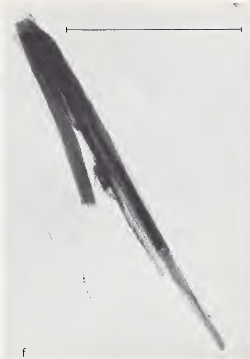
FIGURE 2f. Electron micrograph of hydration products of paste-hydrated C_2S .
