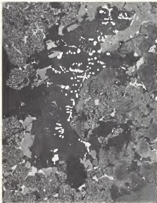
FIGURE 7. Intense disintegration of alite in a specimen bearing calcium sulfide (white, round spots).
