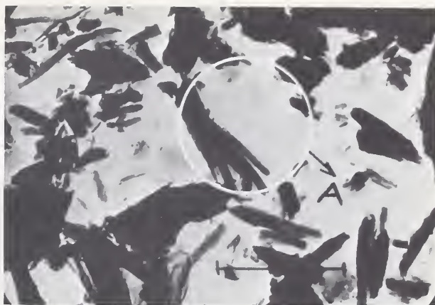
FIGURE 9. Electron micrograph of hydrated \beta\text{-C}_2\text{S} .
