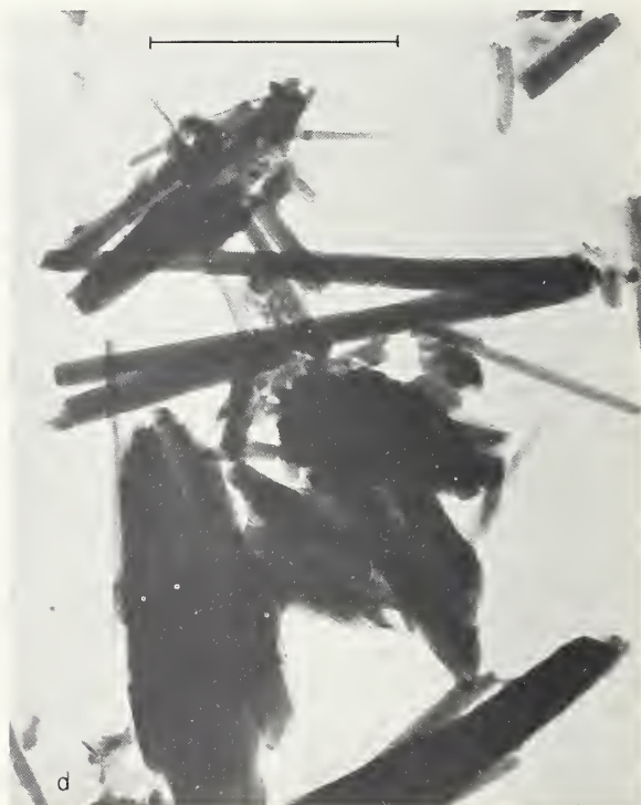
FIGURE 2d. Electron micrograph of hydration products of paste-hydrated C_3S .
