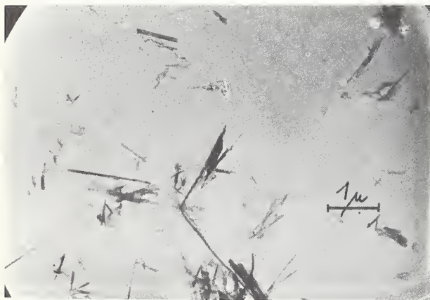
FIGURE 12. Electron micrograph of synthetic tobermorite— 5\text{CaO} \cdot 6\text{SiO}_2 \cdot 5\text{H}_2\text{O} .
