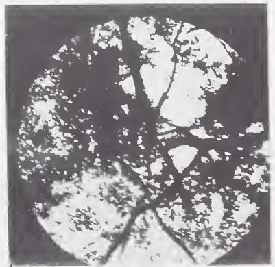
FIGURE 3. Calcium sulfoaluminate formed by interaction of cement clinker with gypsum.
