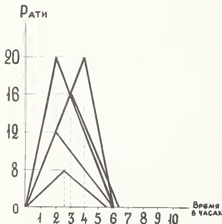
FIGURE 13. "Peak-regime" influence on hardening of cement mortar of the composition 1:3 of plastic consistency. (Ordinate: steam pressure, atm. Abscissa: autoclaving period, hr.)
