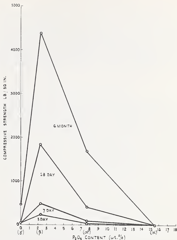
FIGURE 1. Compressive strength (on 1/2'' 1:3 mortar cubes) of preparations on the join C 2 S-C 3 P, showing effect of C 2 S polymorphism.
