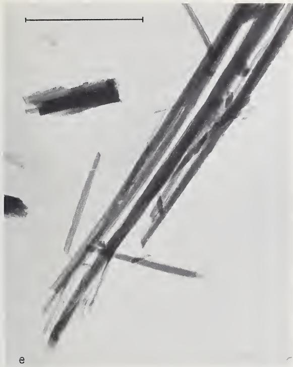
FIGURE 2e. Electron micrograph of hydration products of paste-hydrated C_2S .
