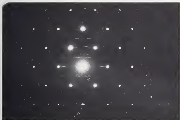
FIGURE 3. Single-crystal diffraction pattern of the reaction product after 4 hr. Crystal lying on (001), b -axis vertical.
