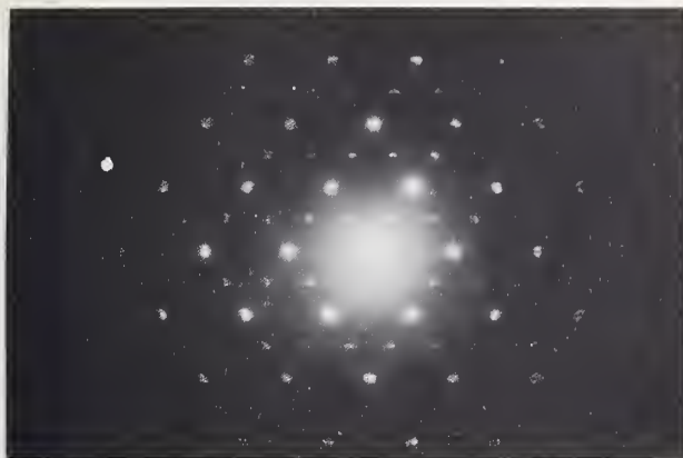
FIGURE 2. Single-crystal diffraction pattern of the reaction product after 3 hr. Crystal lying on (001), b -axis vertical.
