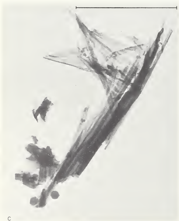
FIGURE 2c. Electron micrograph of hydration products of paste-hydrated C_3S .
