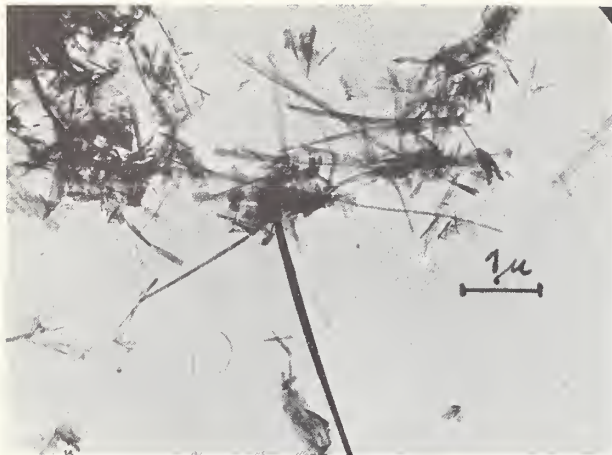
FIGURE 11. Electron micrograph of synthetic tobermorite— 5\text{CaO} \cdot 6\text{SiO}_2 \cdot 5\text{H}_2\text{O} .
