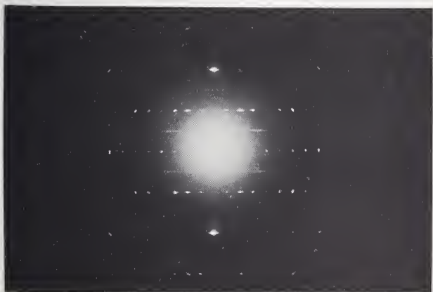
FIGURE 4. Single-crystal diffraction pattern of the reaction product after 5 hr. Crystal lying on (100), b -axis vertical.
