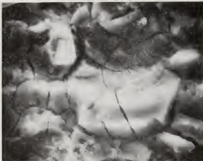
FIGURE 11. "Mud Crack" pattern on surface of stress corrosion crack in alloy 5456-H321, possibly sensitized in service. The features of the mud crack pattern are unrelated to features of the underlying metal. Scanning electron micrograph, magnification 1500X. Photo courtesy of Dr. C. T. Fujii. (From ref. [9])
