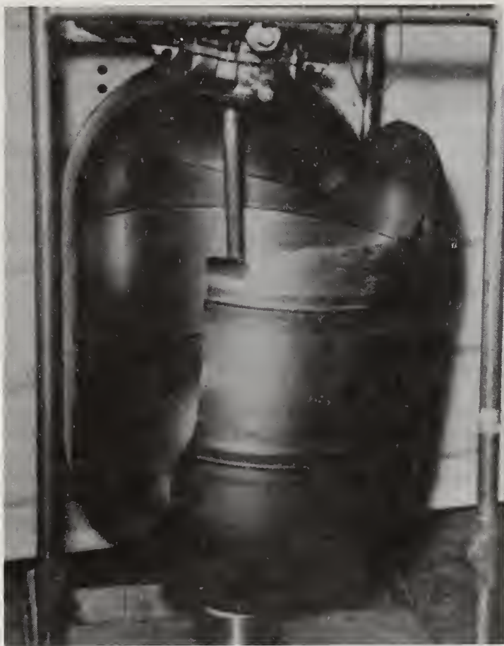
FIGURE 5. Pressure vessel made of Ti-6%Al-4%V which cracked because of N_2 O_4 . Photo courtesy of Dr. L. J. Korb, Rockwell International Space Division.
