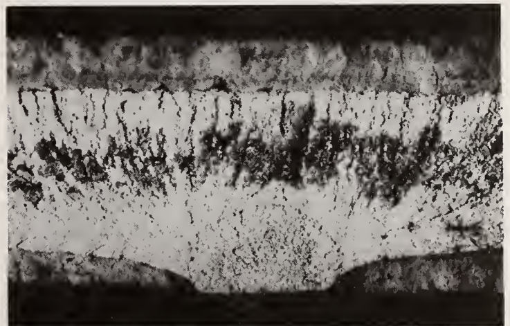
FIGURE 4. Origin of failure of figure 3, enlarged about 15X. Thumbnail-shaped area at bottom is stress corrosion cracking. Brittle fracture chevrons are beginning to develop, radiating from the thumbnail area. Gray bands at top and bottom are shear lips. Dark areas on brittle fracture are rust. Photo by D. Price.
