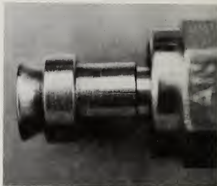
FIGURE 1. SCC in AISI type 303 stainless steel sleeve in service in the marine atmosphere near windward surf at Cape Kennedy. Magnified 3X. This sort of cracking of austenitic stainless steel at room temperature is rare. A similar steel but without the extra sulfur or selenium of 303 would probably not have cracked. Courtesy of Mr. J. D. Morrison, NASA.
