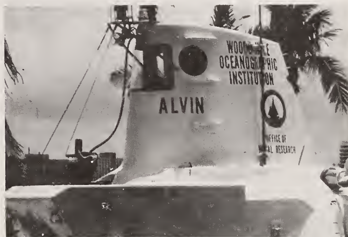
FIGURE 1. The research submersible ALVIN, which is equipped with a pressure hull made of Ti-6%Al-2%Cb-1%Ta-0.8%Mo and with 15 buoyancy spheres made of low oxygen Ti-6%Al-4%V. It is possible to crack both these alloys in the laboratory at high K levels, but the design and fabrication of the hull and buoyancy spheres were such that the vehicle has performed satisfactorily in the sea.
