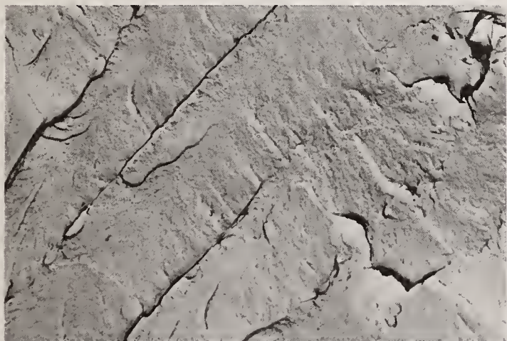
FIGURE 7. Intergranular cleavage-like SCC fracture of Ti-8%Al-1%Mo-1%V in salt water. Note local plasticity toward right side. Electron fractograph, magnification 6000X. Courtesy of Mr. D. A. Meyn.
