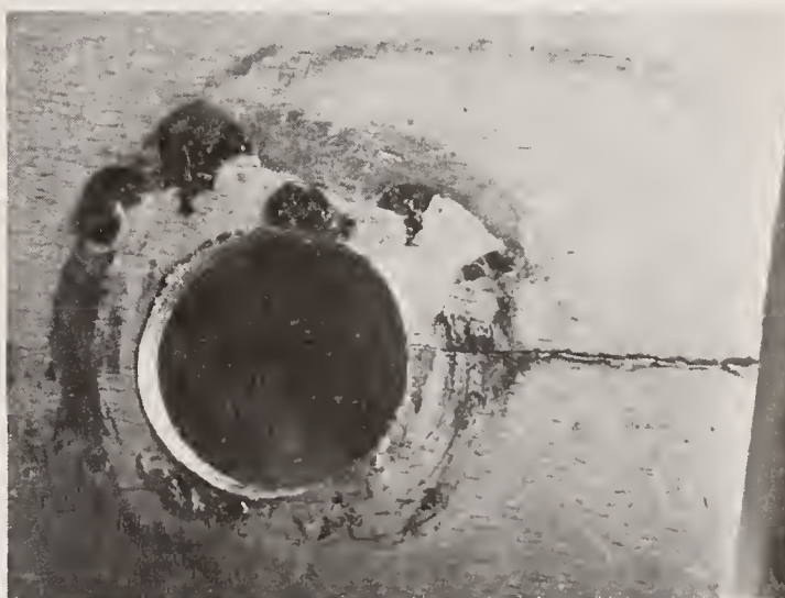
FIGURE 7. SCC in end of extruded tube of 7075-T651, C-L crack plane. Terrestrial failure of Apollo Program Lunar Excursion Module component, stressed by taper pin which was driven into the hole shown. Cautious practice does not permit such pins stressing the vulnerable texture unless the -T73 temper is used. Magnified 3X. Courtesy of Mr. C. D. Beachem.
