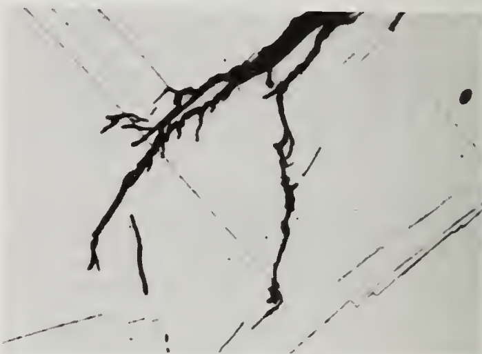
FIGURE 6. High magnification (900X) photomicrograph of transgranular SCC produced in the laboratory. AISI type 304 stainless steel. Courtesy of Dr. J. Kruger, National Bureau of Standards.
