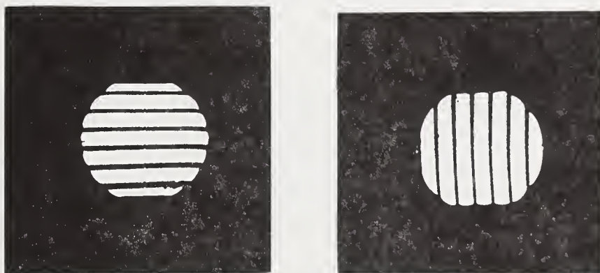
Figure 2. Typical gage block fringe pattern.
