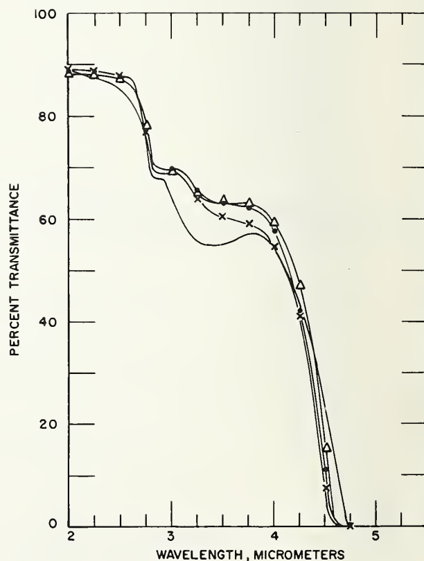
FIGURE 28. Spectral transmittance of 2-mm thickness of glasses containing 26 mol percent of BaO. × F705, ● F707, Δ F709, — F716.
