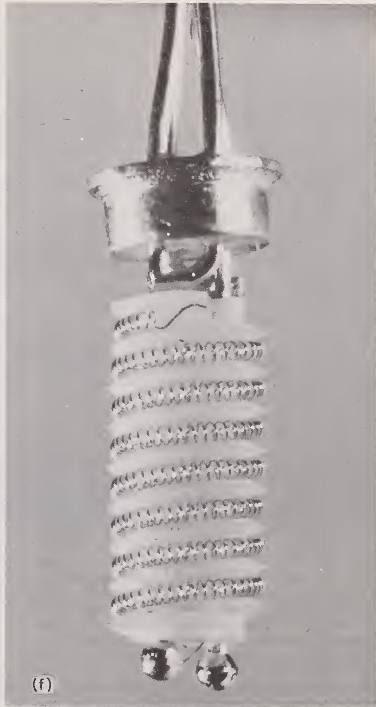
FIGURE 2—Continued. Construction of the coils of some thermometers.
