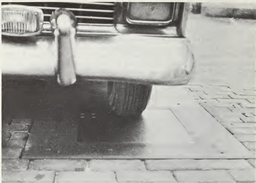
FIGURE 7.2.17. Road platform tire tester having the possibility of measuring three perpendicular forces of a tire moving over the platform.
