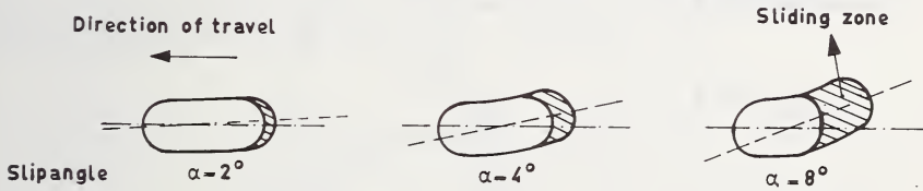
FIGURE 7.3.17. The sliding zone at the rear of the contact area.
