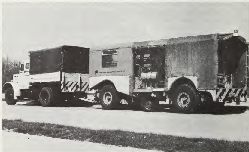
FIGURE 7.2.8. Towed trailer road tests with a six-component tire tester. The test wheel is mounted in the airsprung trailer.
