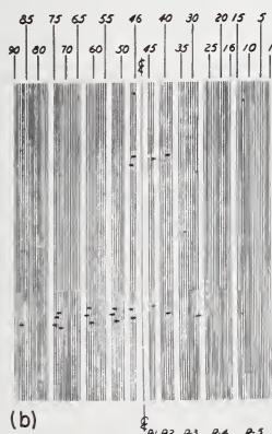
FIGURE 1.3.51. Break location for a 22% cotton-78% dacron yarn model with asymmetrically located low elongation elements. TM=1.09 .
