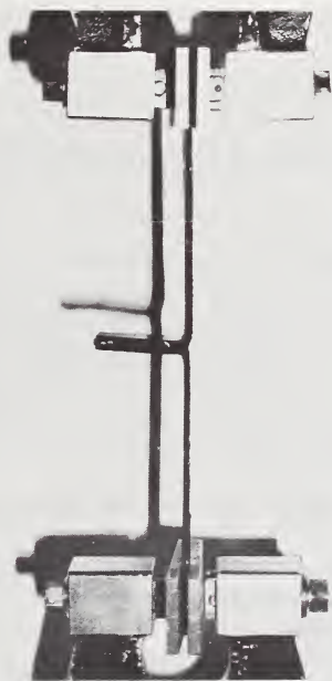
FIGURE 1.4.72. Testing arrangement for two-ply strip test.
