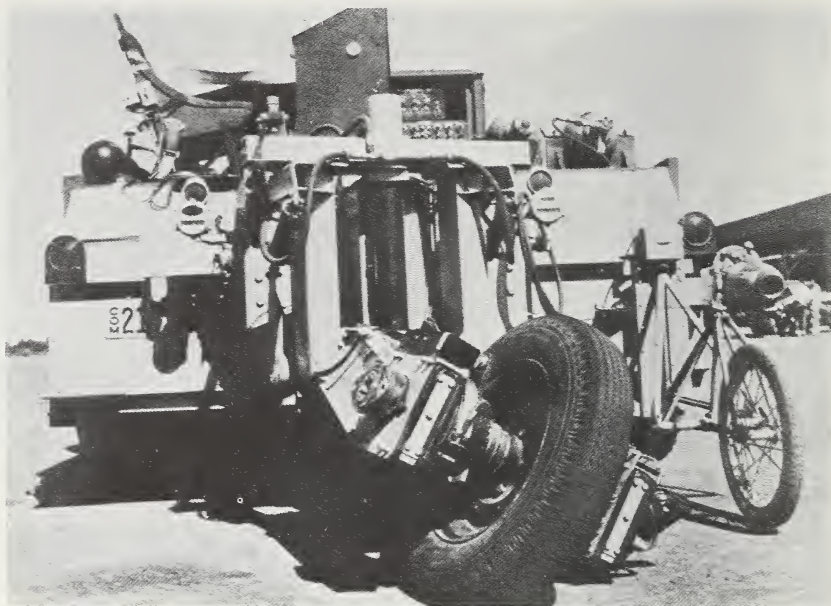
FIGURE 7.2.7. Single wheeled trailer behind a truck for measuring tire characteristics. A fifth wheel is also shown for accurate slip angle measurements.
