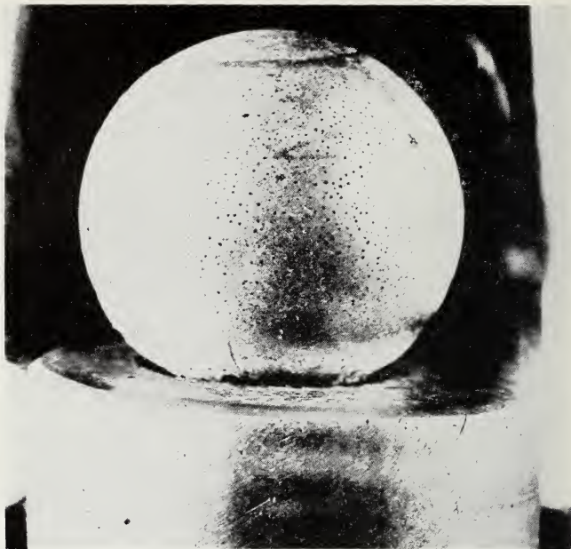
FIGURE 7. Copper spherical single crystal pitted by bombardment with oxygen atoms.
