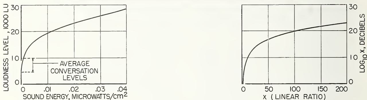
FIGURE 1. As the curve at the left shows, if the power of a sound is increased, the sensation of loudness perceived by a listener does not increase as rapidly as the increase in power.
