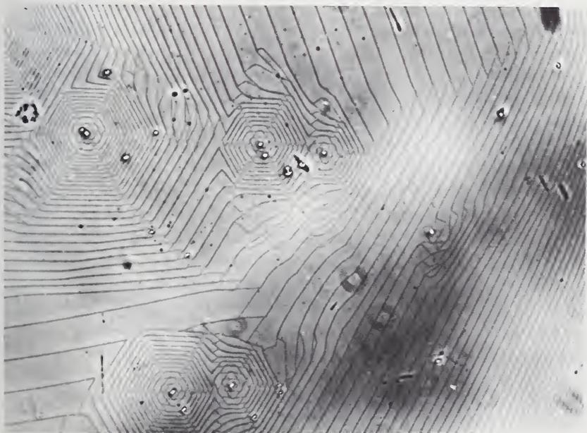
Figure 17. Etch pattern on the *c*-face of silicon carbide. Pits located at the centers of growth spirals, as well as pits located elsewhere can be seen. The growth spirals have become visible as a consequence of preferential attack along the growth steps. Single steps are only 7 Å high.
