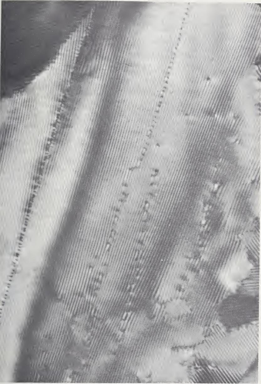
Figure 72. Lattice fringes in tantalum pentoxide. Note the presence of dislocations and sub-grain boundaries. Courtesy Spyridelis.
