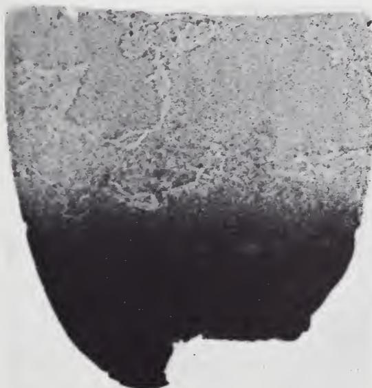
Figure 1. Autoradiogram of Al-Cu 4; ingot;  $\times 3$ .
