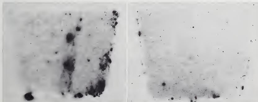
Figure 3. Autoradiograms of aluminum block cut using: a) ordinary steel turning tool; b) turning tool made from tungsten carbide.
