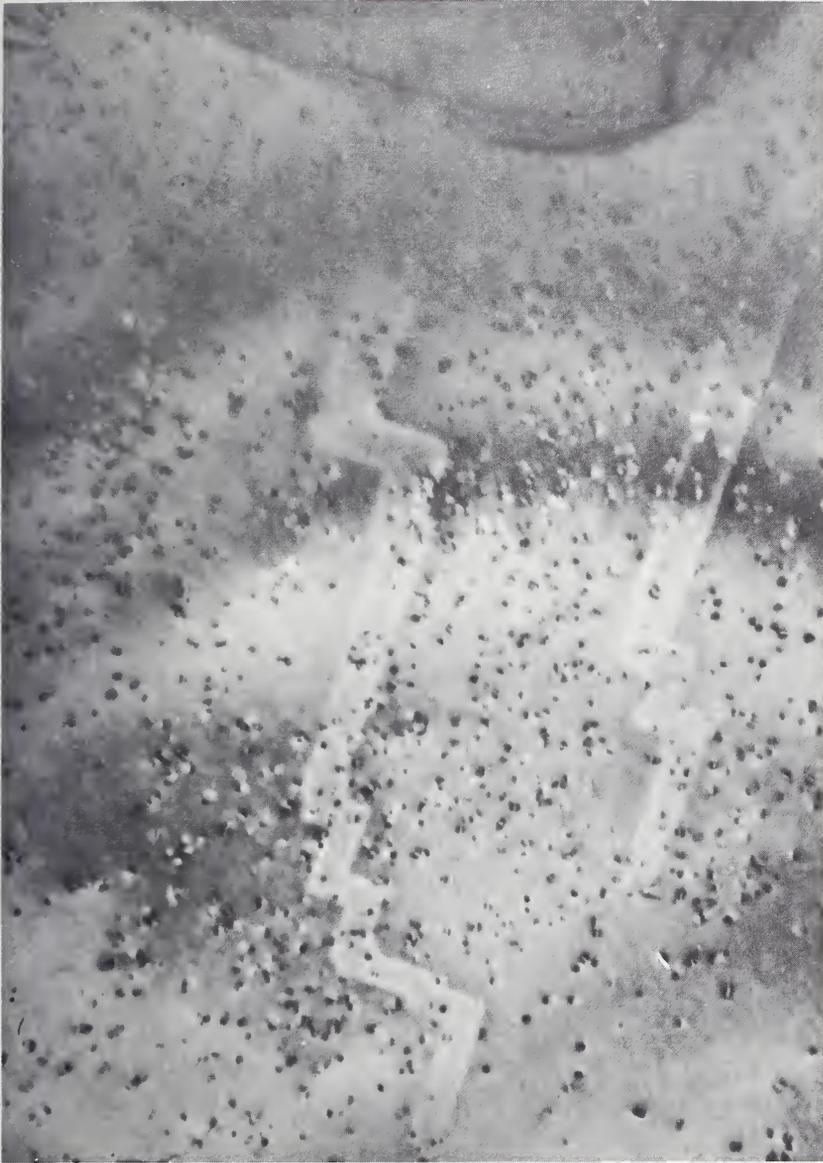
Figure 57. Cross slip pattern observed in quenched aluminum foil. From the slip traces the foil thickness can be computed. Anomalously wide images due to loops close to the surface can be observed also. Courtesy of R. Cotterill.
