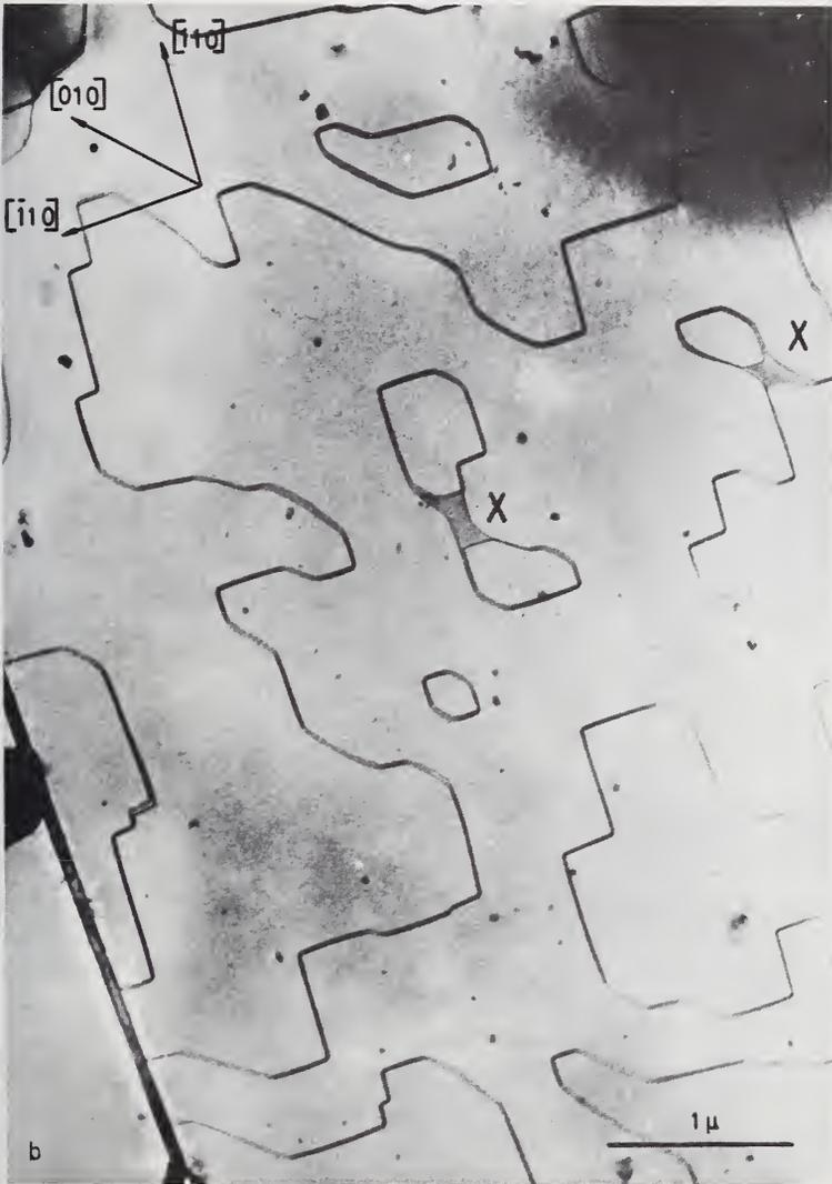
Figure 45(b). Antiphase boundaries in Tealite ( $\text{SnPbS}_2$ ). Courtesy Marinkovic.
