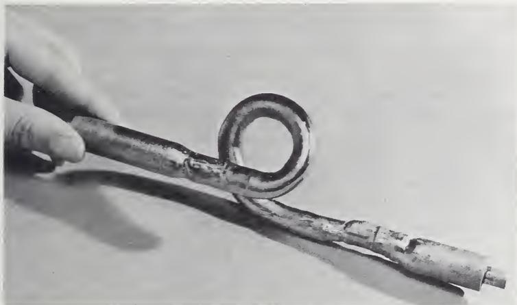
Figure 14. Ductility of pure Be. After Schaub and Cabane, *Compt. Rend.* **257**, (2), 444 (1963).
