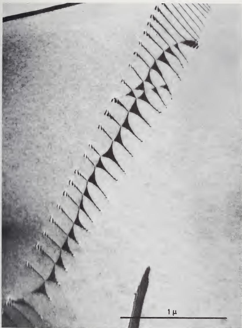
Figure 56. Network of extended and contracted nodes in a copper-gallium alloy.
