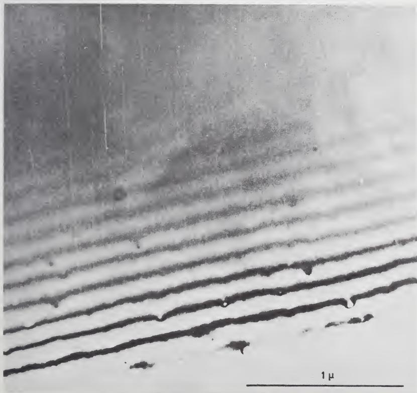
Figure 28. Thickness contours in a wedge shaped silicon foil.
