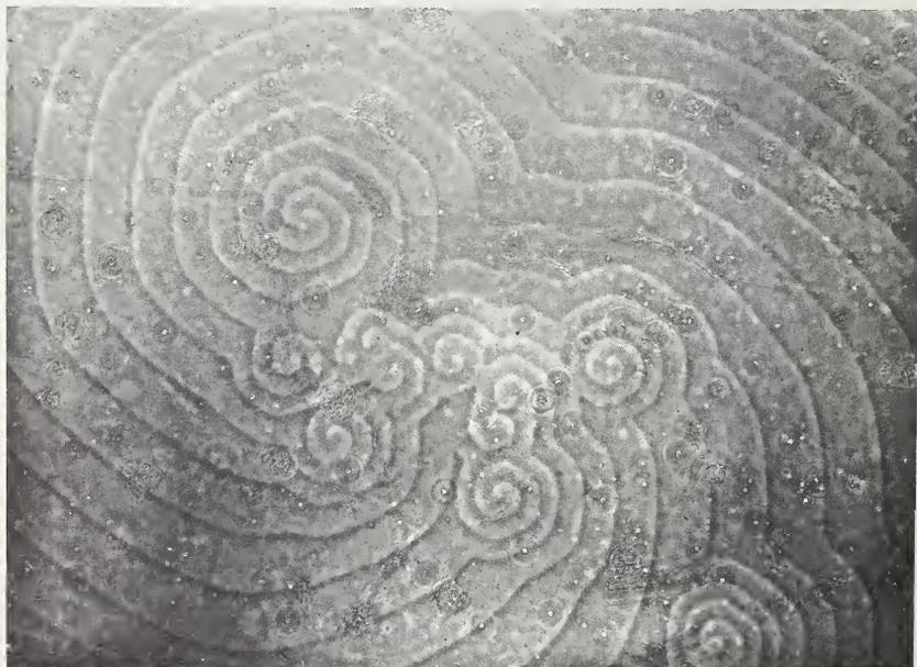
Figure 15. Growth promoted by a number of spirals of the same sense originating in a group of dislocations with components perpendicular to the  $c$ -face of the same sign. The step heights are  $13 \text{ \AA}$ .
