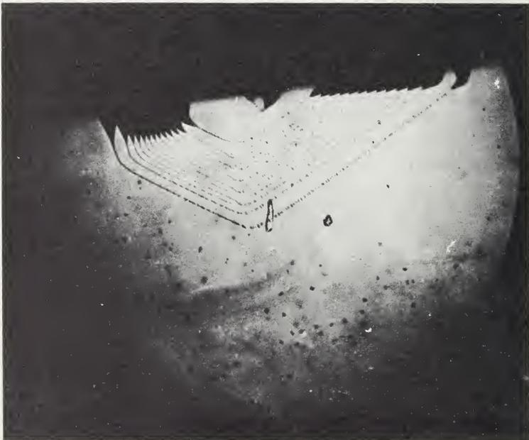
Figure 22. Termination of dislocations in etch pits. Copper has been precipitated on silicon dislocations, with photograph taken by transmitted infrared. After Dash [19].
