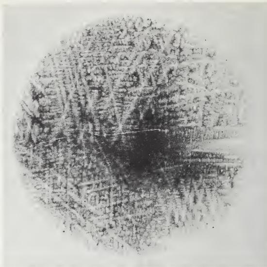
Figure 2. Autoradiogram of Al-Ni 0.3; ingot;  $\times 8$ .
