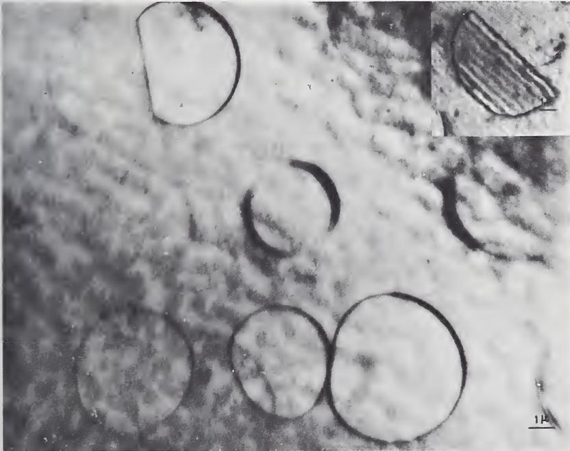
Figure 35. Loops in the basal plane of zinc. Two types of images are visible. The Burgers vector of the loops is inclined with respect to the basal plane. The inset shows stacking fault fringes for loops which are inclined with respect to the foil plane. Courtesy Stals.
