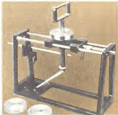
NBS-Brungraber Portable Slip Resistance Tester developed to measure the slipperiness of surfaces.
