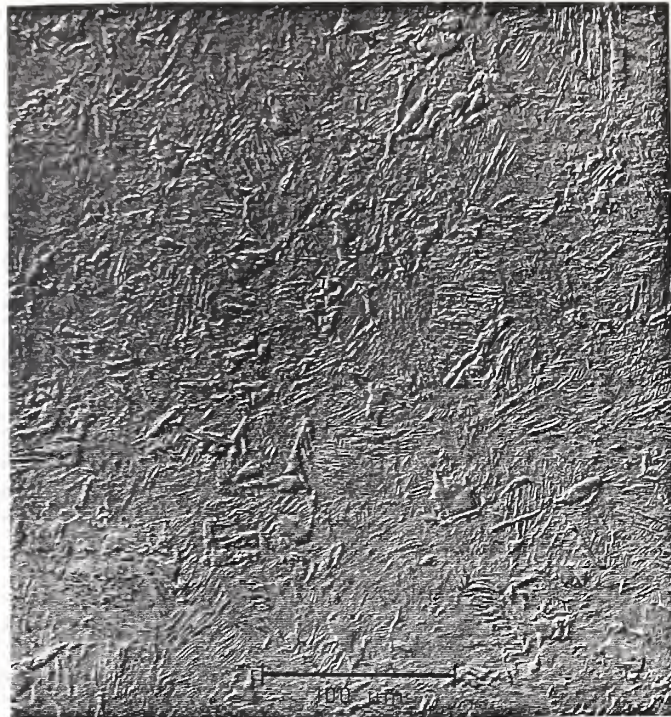
Figure 3. Representative microstructure of a wire from one of the outside strands of the 6 x 7 wire rope sample. Etchant: Glyceregia X 250
