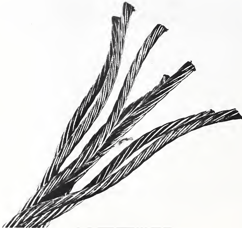
Figure 8. Broomed end of a specimen of the 6 x 7 wire rope.
