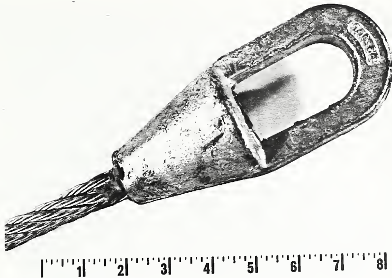
Figure 9. Terminal configuration for tensile tests (scale in inches).
