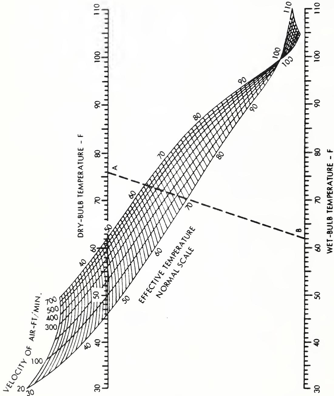
**HOW TO USE THE CHART:** Draw line A-B through measured dry-bulb and wet-bulb temperature. Read effective temperature or velocity at desired intersections with line A-B. **EXAMPLE:** Given 76 F db and 62 F wb, read: 69 ET at 100 fpm velocity, or 340 fpm required for 66 ET.
