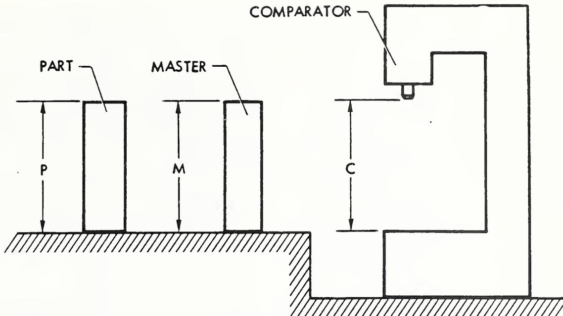
FIG. 11 The three elements of a length-measuring system.
