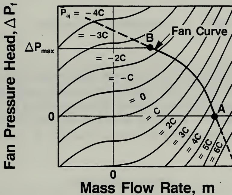
Figure 6. Graphical solution of mass flow through a fan-resistance system
