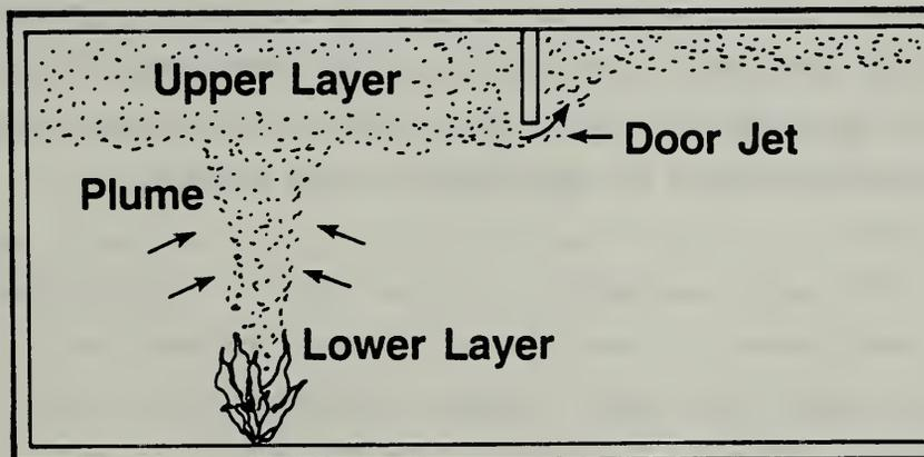
Figure 1. Stratified smoke flow as simulated by zone fire models
