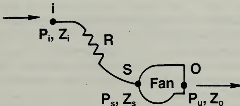
Figure 2. Schematic diagram of a simple fan-resistance system
