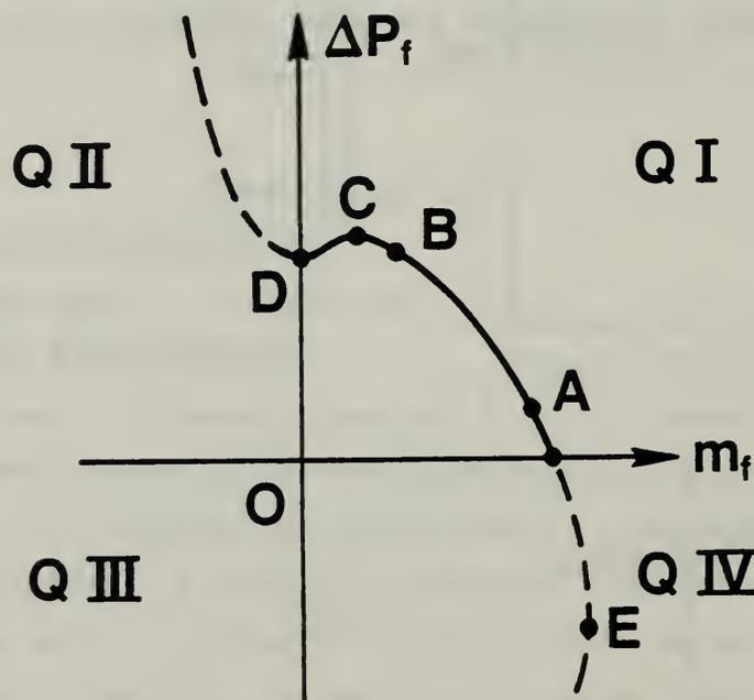
Figure 4. Typical performance of a constant speed fan
