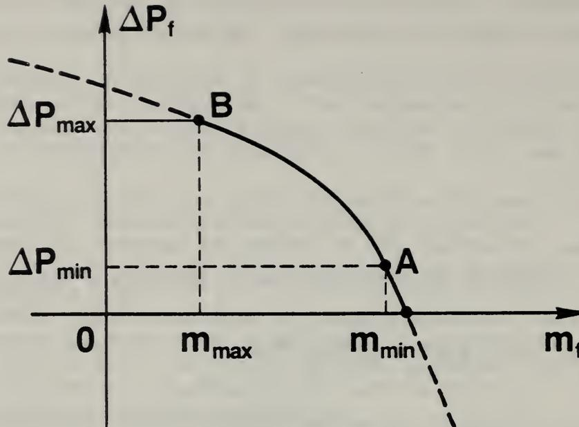
Figure 5. Idealized fan curve used in FANRES
