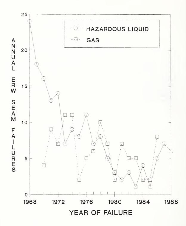
Figure 1. Annual Number of ERW Seam Failures in Hazardous Liquid Transmission Lines and Natural Gas Gathering and Transmission Lines During the Period 1968-1988 (15).
