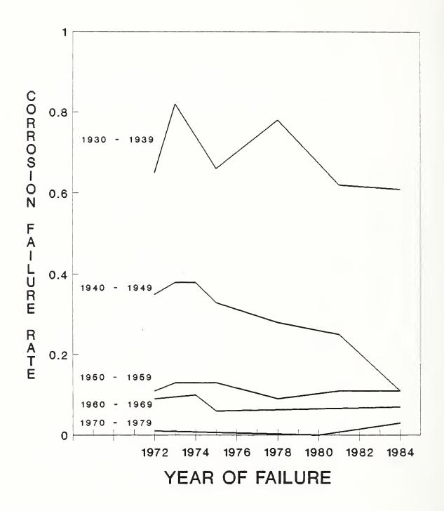
Figure 3. Annual Rates of Corrosion Failures (number per year per 1000 miles of pipeline) in Natural Gas Gathering and Transmission Lines for the Period 1970-1984 Classified by Decade of Construction (16).
