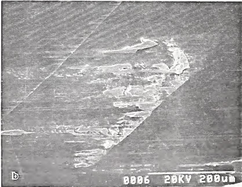
Fig. 29. Patches of transferred Ag on Ni flat (a) near beginning of track and (b) near end of track.
