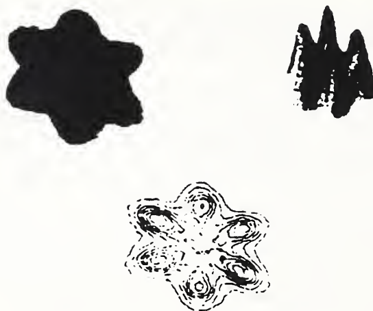
Fig. 3.1. F^- ESDIAD patterns for monolayer of PF_3 adsorbed at 110 K on Ru(0001) and annealed to 273 K. Upper left: F^- ESDIAD image as it appears on phosphor screen of ESDIAD apparatus. Upper right: Perspective plot of F^- ESDIAD, obtained using digital video image processor. Bottom: Intensity contour map of F^- ESDIAD.
