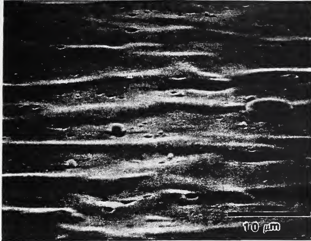
Figure 4. The spherical inclusions are MnSiO_3 type inclusions typically found in stainless steel welds. The more angular, dark inclusions were rich in Cr and/or Ti.
