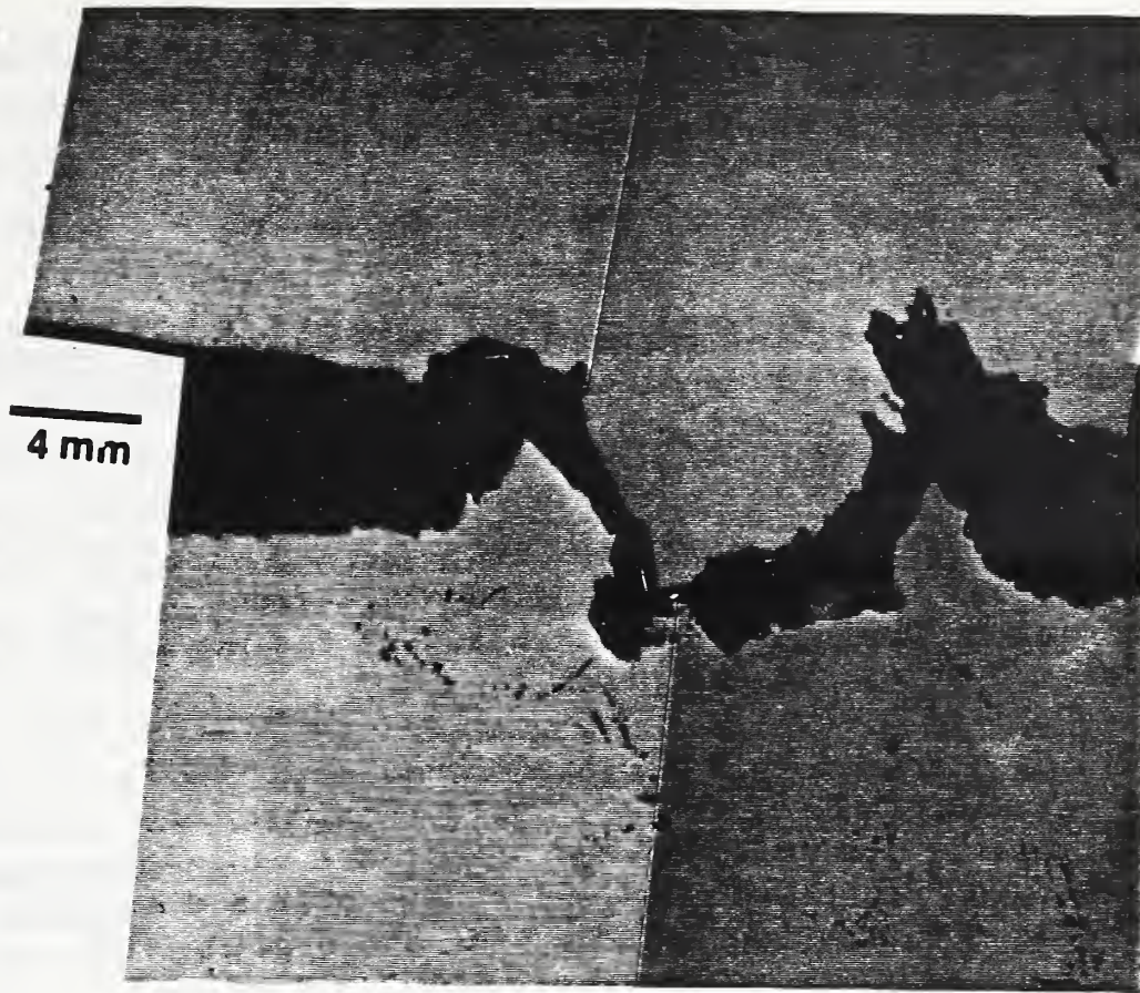
Figure 6. Section of crack tip in alloy #3 with J_a > J_{Ic} showing the angled path of initial crack growth.
