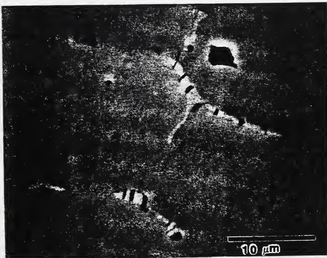
Figure 9. In the 1S tensile specimen, deformation of the austenitic matrix often resulted in the fracture of ferrite particles and sometimes cracks at inclusion sites were observed. The textured appearance of the matrix is due to plastic flow.
