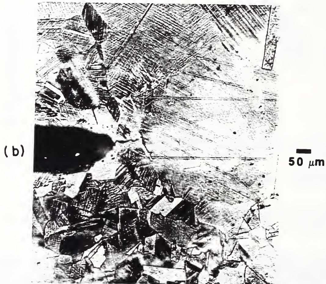
Figure 4 Etched microstructure of the area around the blunted crack tip in alloy 2. The test was interrupted at an applied energy = 0.35 J_{Ic} .
