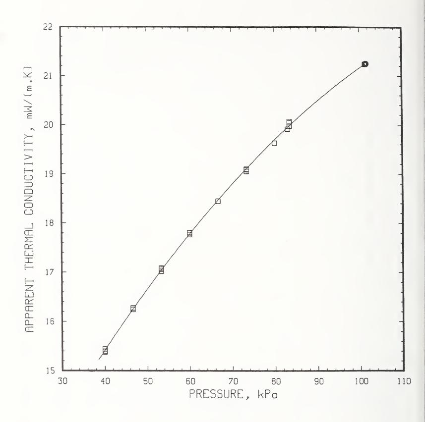
Figure 5. Extrapolated correlation of thermal conductivity with with pressure, eq(2), estimating thermal conductivivity of microporous fumed-silica insulation at sea-level atmospheric pressure (101.3 kPa) as indicated by the open circle at the top. Mean temperature of specimens is 318 K.
