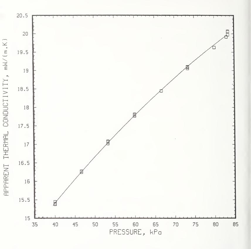
Figure 3. Thermal conductivity of a pair of microporous fumed-silica insulation boards with a mean density of 301 g/m3, at a mean temperature of 318 K (45°C). Measurements were performed in air at ambient humidity and at pressures varying from 40 to 83.5 kPa (300 to 626 Torr). The solid line was calculated from eq(2).
