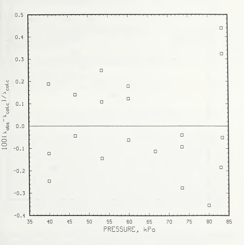
Figure 4. Deviations of thermal conductivity of microporous fumedsilica specimens from values calculated with eq(2).
