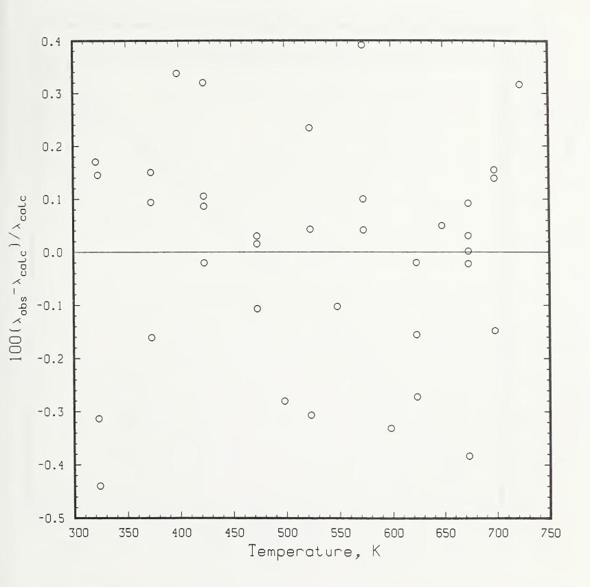
Figure 2. Deviations of thermal conductivity of microporous fumedsilica specimens from values calculated with eq(1).
