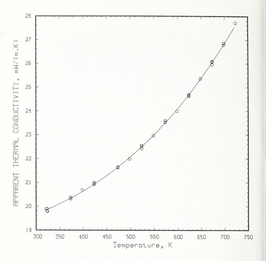
Figure 1. conductivity of a Thermal pair of microporous fumedsilica insulation boards with a mean density of 301 kg/m3, temperatures from 321 to 723 K (48 450oC). at mean to Measurements were performed in air at ambient humidity and pressure of 83.6 kPa (627 Torr) using the NIST/B at а high-temperature guarded hot plate. The measurement bias in values of Kmeas is estimated to be 1.5% at 330 Κ, and 2.5% 720 K. at The solid curve represents values of Kcalc, obtained using eq(1).
