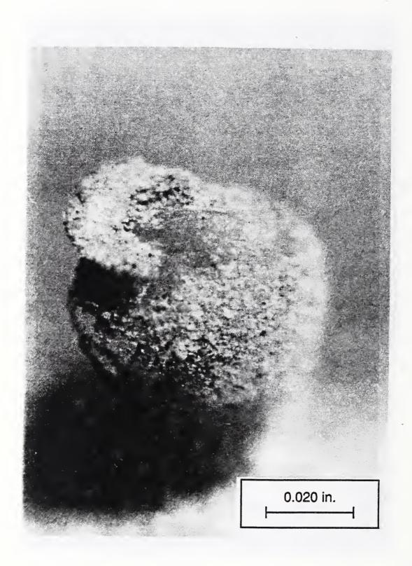
Figure 16. Specimen 5, Sand Grain Adhered to Lower Wire, 45°-Viewing Angle. (Scale is Approximate).
