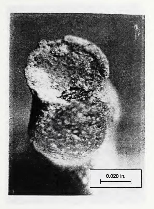
Figure 3. Specimen 1, Sand Grain Adhered to Lower Wire, 45° Viewing Angle (Scale is Approximate).
