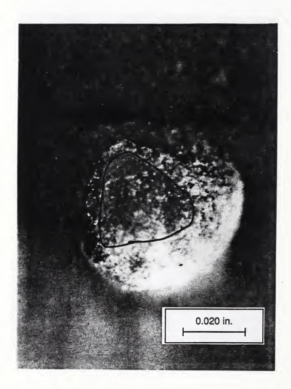
Figure 18. Specimen 5, Sand Grain Adhered to Upper Wire, Estimated Planar Bond Failure Surface Area (Used in Table 1) Shown by Enclosed Area, 90°-Viewing Angle.
