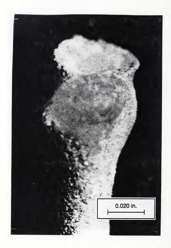
Figure 4. Specimen 1, Sand Grain Adhered to Lower Wire,  $0^{\circ}$ -Viewing Angle.
