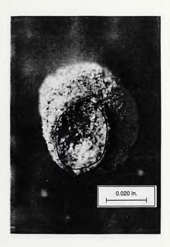
Figure 9. Specimen 3, Sand Grain Adhered to Lower Wire, Estimated Planar Bond Failure Surface Area (Used in Table 1) Shown by Enclosed Area, 90°-Viewing Angle.
