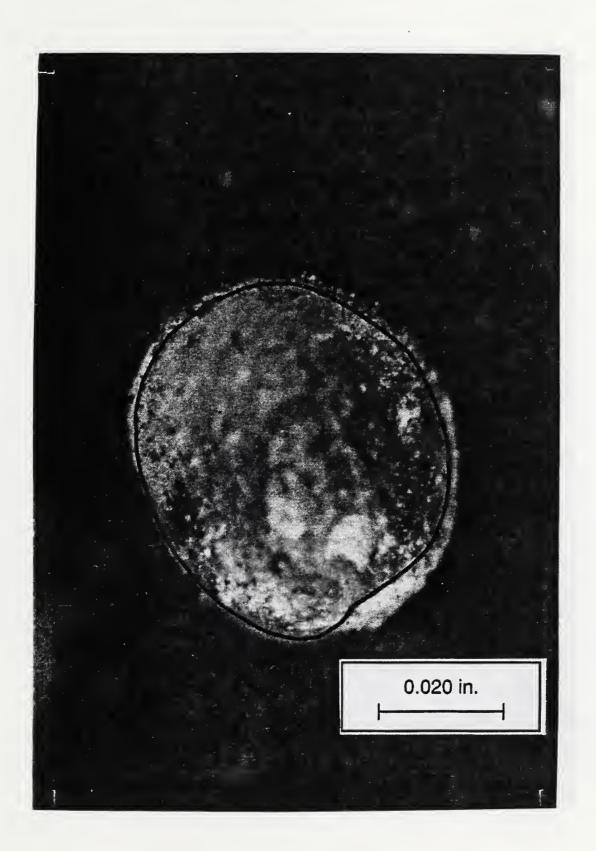
Figure 5. Specimen 1, Sand Grain Adhered to Upper Wire, Estimated Planar Failure Bond Surface Area (Used in Table 1) Shown by Enclosed Area, 90°-Viewing Angle.
