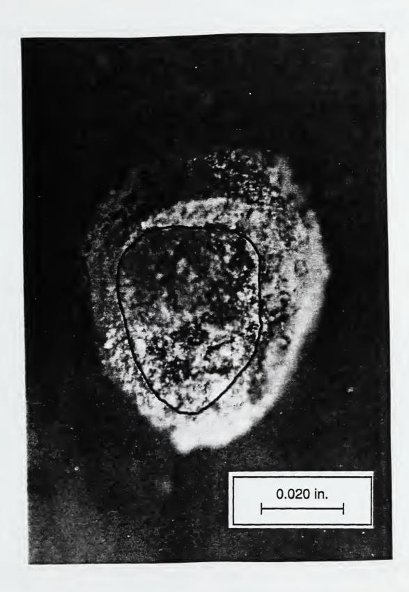
Figure 21 Specimen 6, Sand Grain Adhered to Upper Wire, Estimated Planar Bond Failure Surface Area (Used in Table 1) Shown by Enclosed Area, 90°-Viewing Angle.
