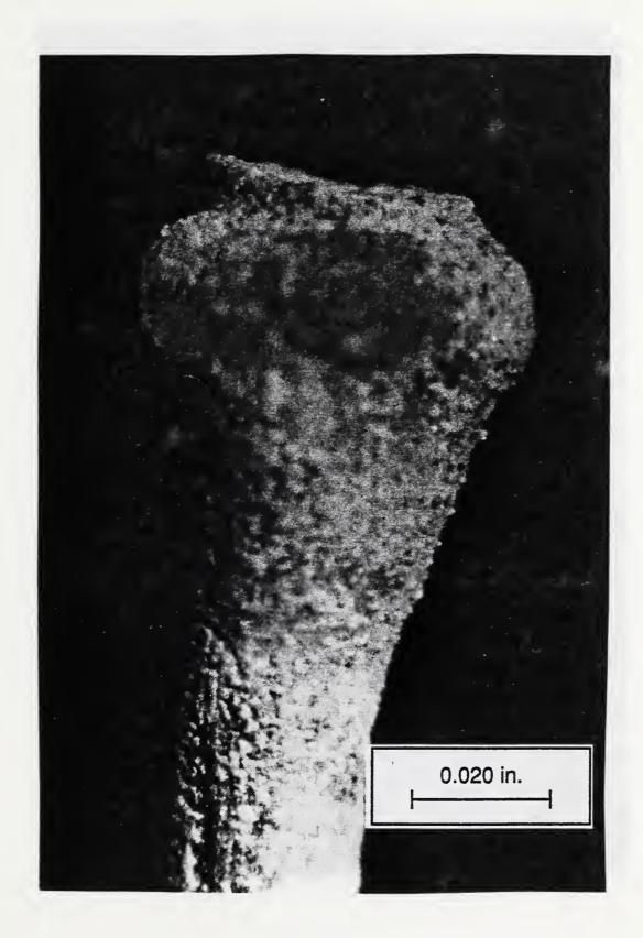
Figure 11. Specimen 3, Sand Grain Adhered to Lower Wire,  $0^{\circ}$ -Viewing Angle.
