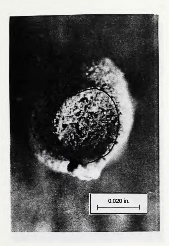
Figure 13. Specimen 4, Sand Grain Adhered to Lower Wire, Estimated Planar Bond Failure Surface Area (Used in Table 1) Shown by Enclosed Area, 90°-Viewing Angle.
