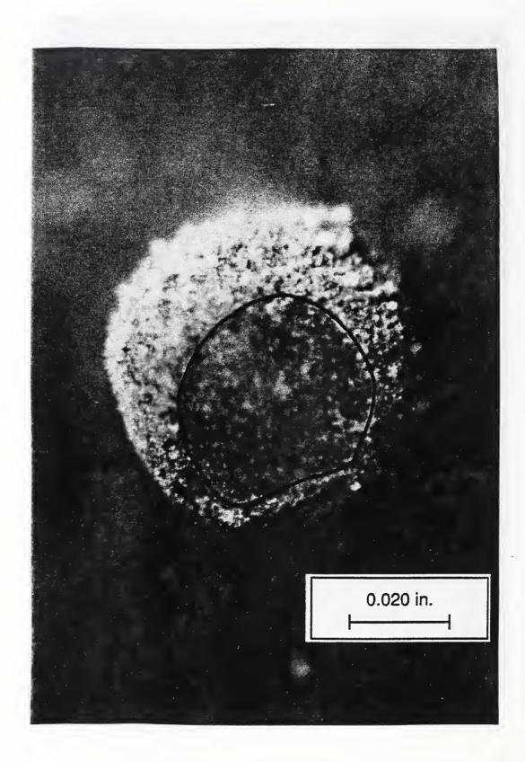
Figure 14. Specimen 4, Sand Grain Adhered to Upper Wire, Estimated Planar Bond Failure Surface Area (Used in Table 1) Shown by Enclosed Area, 90°-Viewing Angle.
