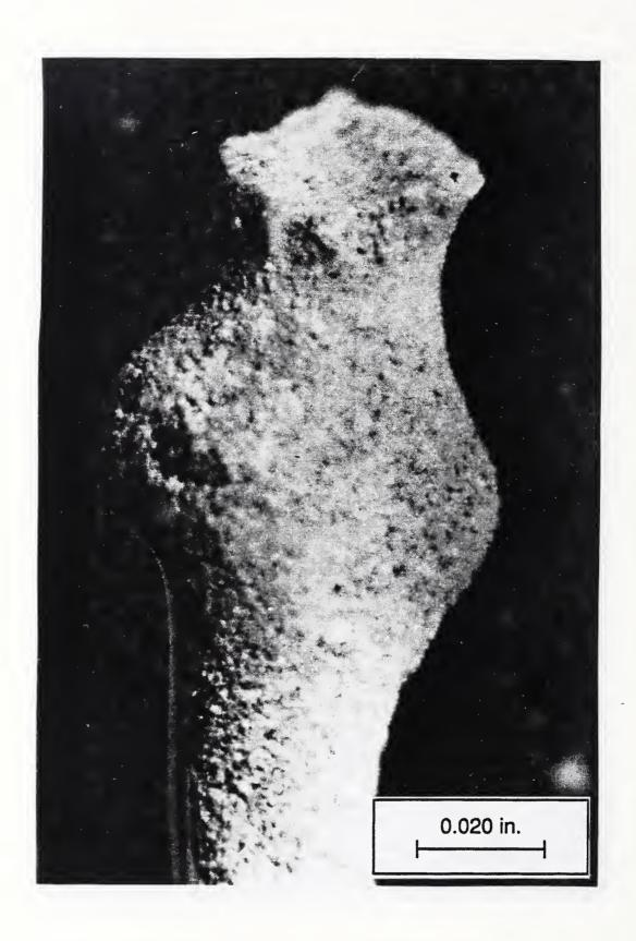
Figure 20. Specimen 6, Sand Grain Adhered to Lower Wire,  $0^{\circ}$ -Viewing Angle.
