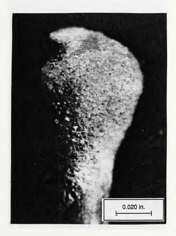
Figure 17. Specimen 5, Sand Grain Adhered to Lower Wire, 0°-Viewing Angle.
