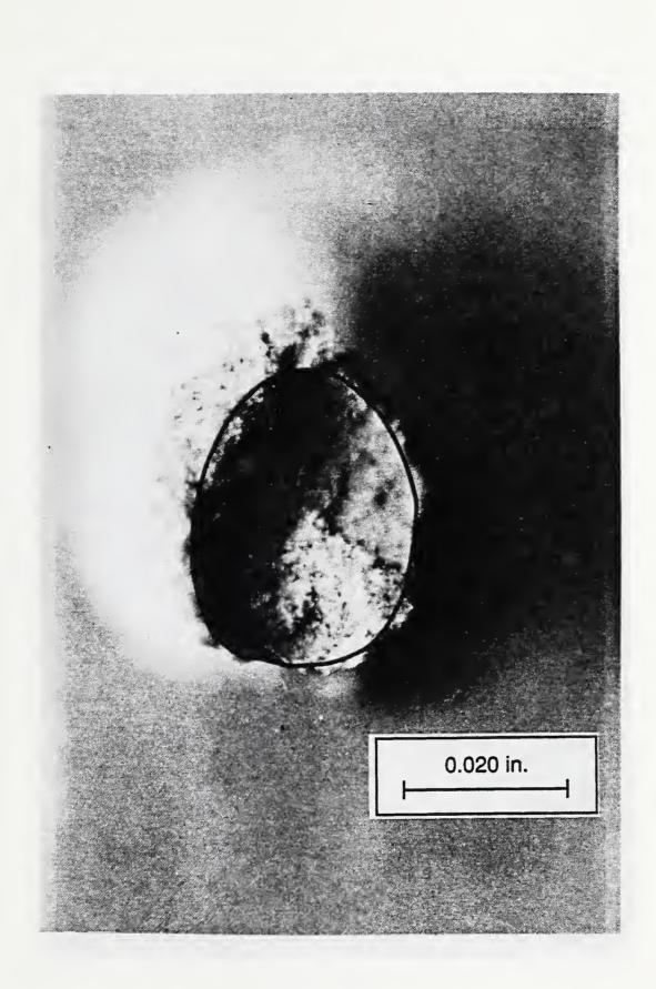
Figure 19. Specimen 6, Sand Grain Adhered to Lower Wire, Estimated Planar Bond Failure Surface Area (Used in Table 1) Shown by enclosed Area, 90°-Viewing Angle.
