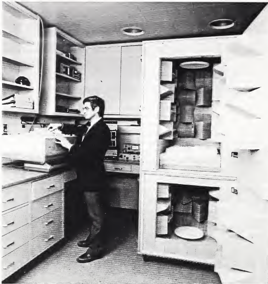
Fig. 4 Photograph of the test chamber with a sample basket installed. The scientist is measuring the thickness of another sample, which is resting on a digital balance.
