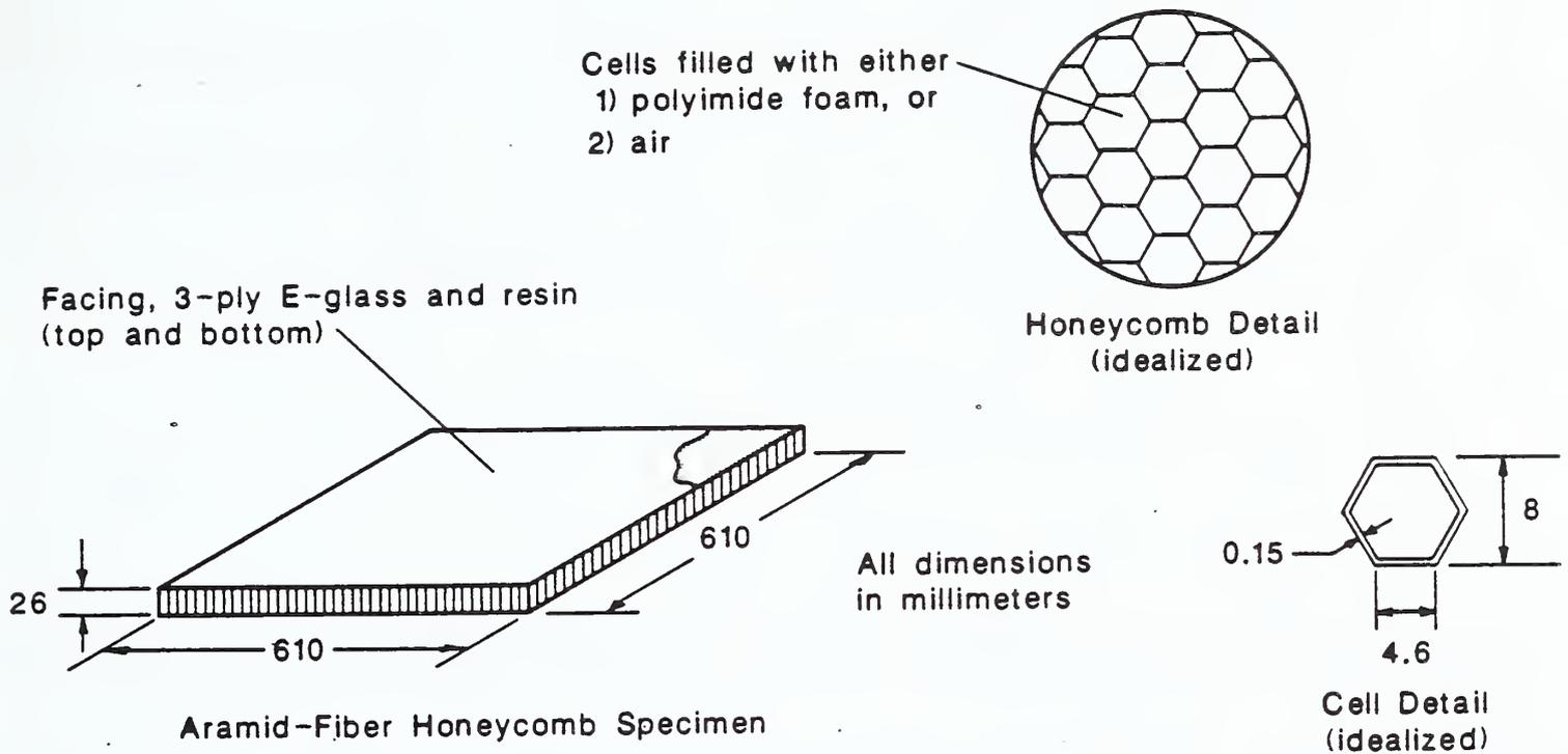
Fig. 3. a) Honeycomb structure of the aramid-fiber honeycomb specimens. Dimensions of the specimen are nominal.
