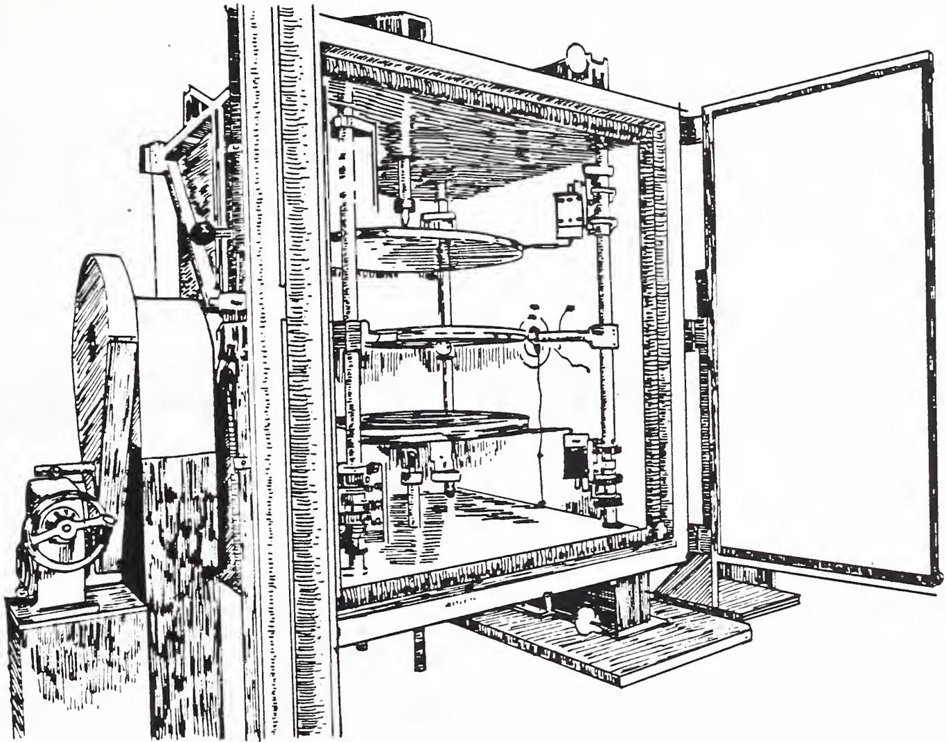
Fig. 1. The NBS 1-metre Guarded Hot Plate.
