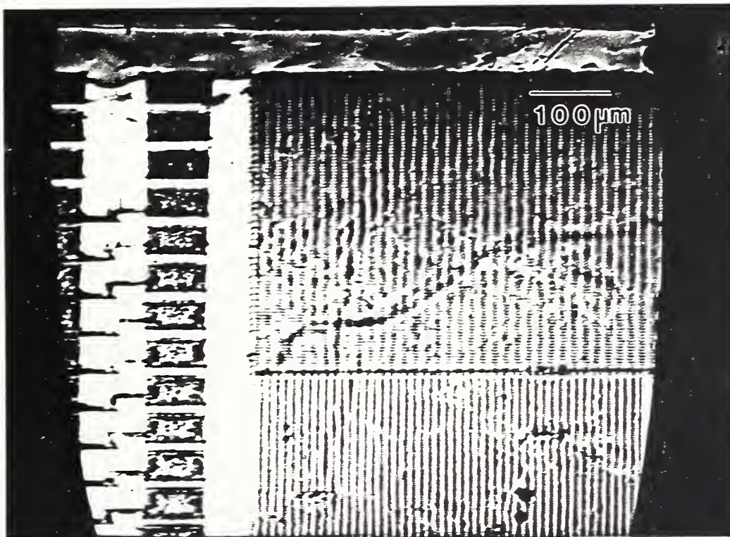
Figure 5a. (400) diffraction image in the surface reflection geometry taken from a device on a gallium arsenide (100) substrate at 9.3 KeV, using an x-ray image magnifier, 30 X.
