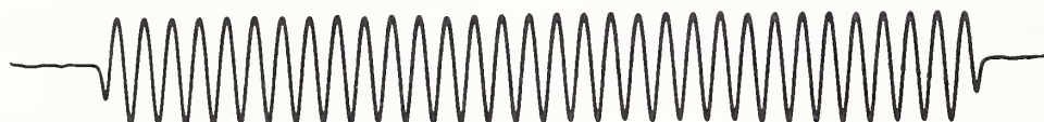
Figure 1. Profilometry scans of a 1.0 \mu\text{m } R_a sinusoidal aluminum surface by (a) a contacting stylus, and (b) a noncontacting ultrasonic echo-amplitude technique.
