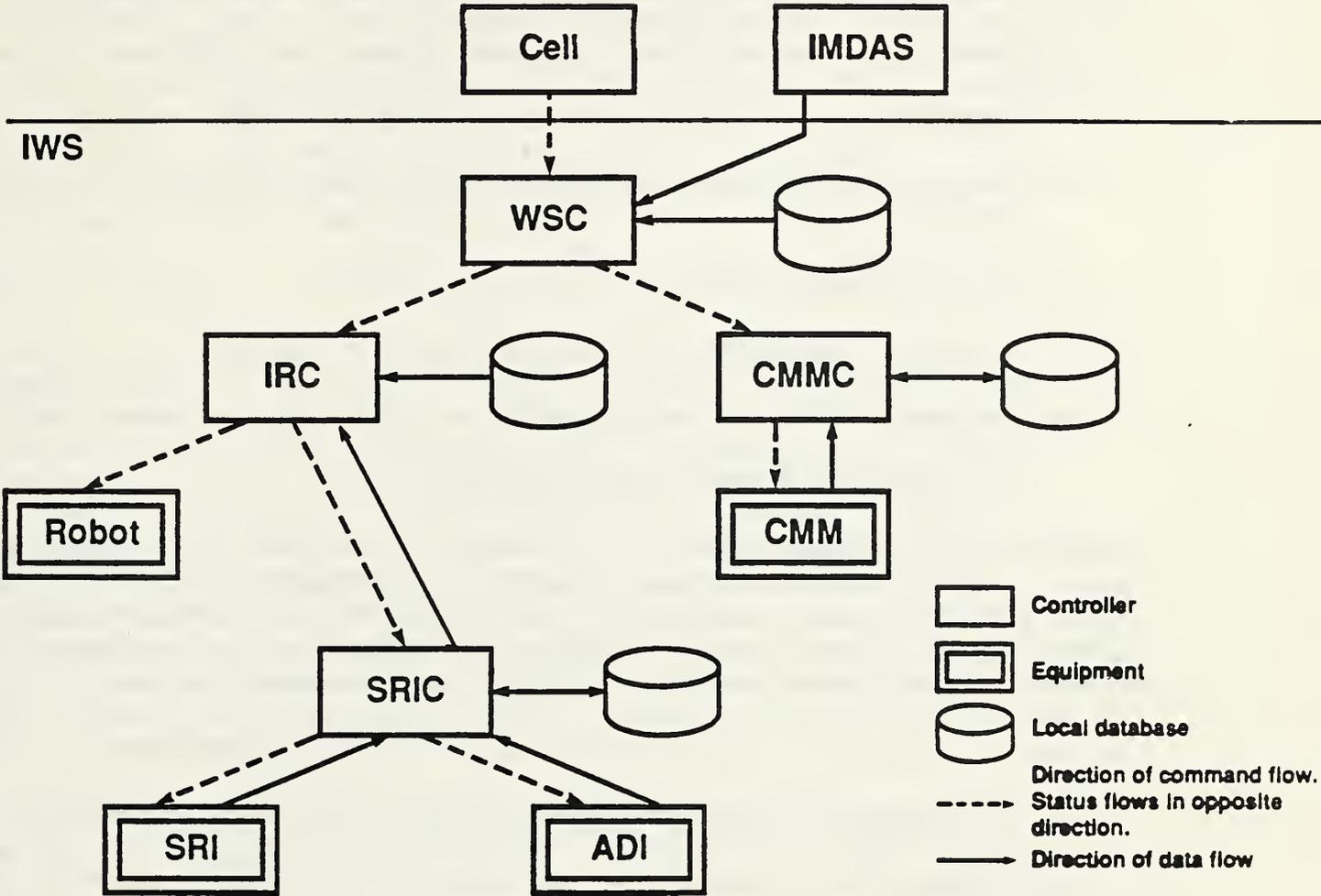
Figure 4. Logical architecture of the IWS.
