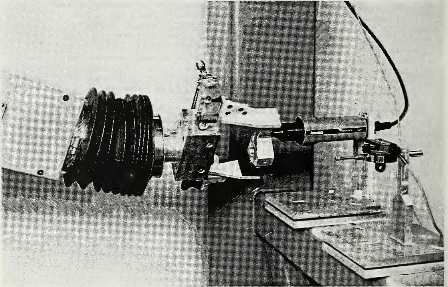
Figure 1. Photograph showing the IWS robot positioning a part in front of the SRI
