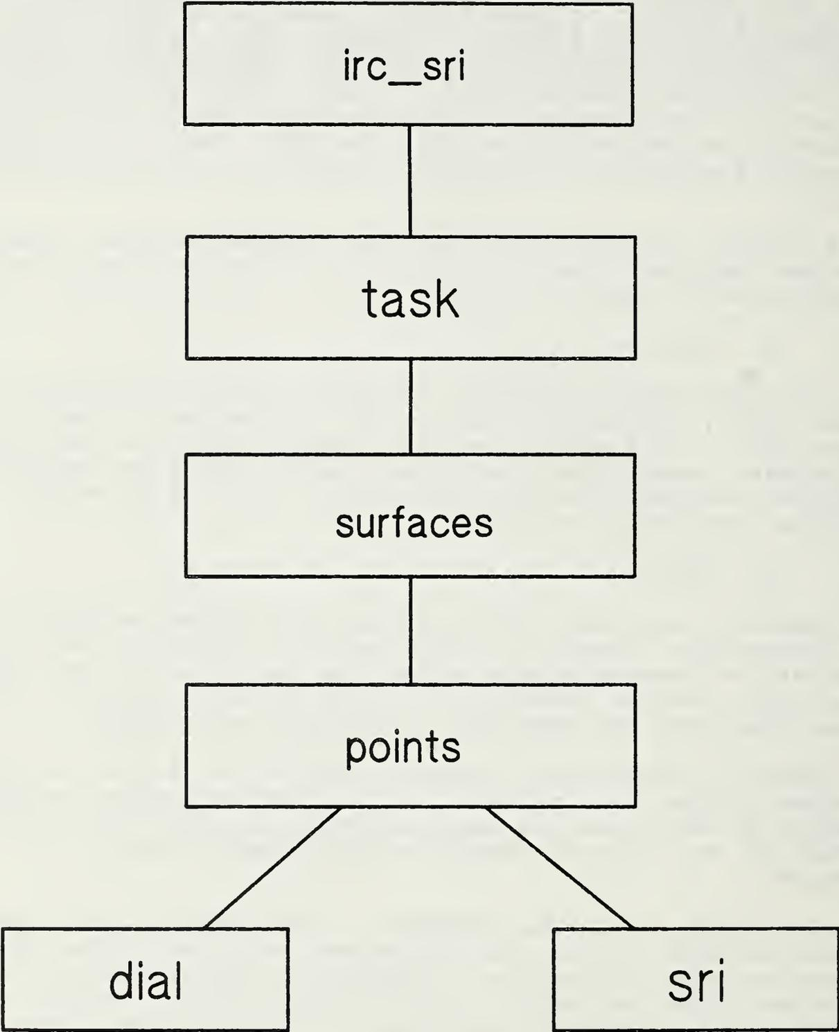
Figure 8. Control Levels for the SRI Controller
