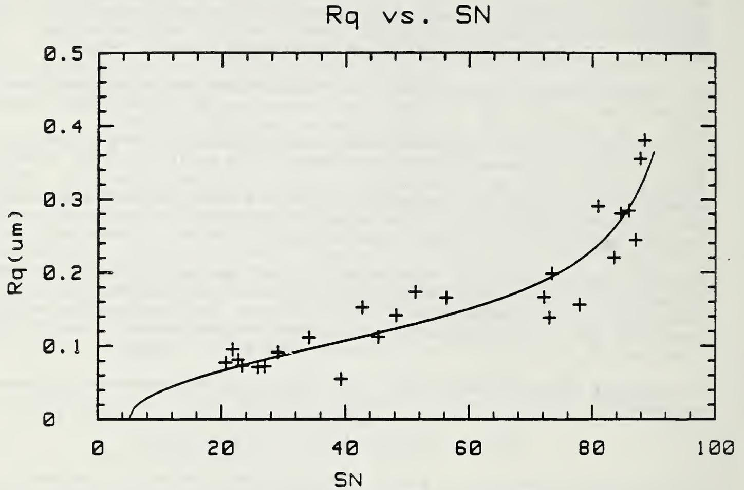
Figure 7.  $R_q$  values measured with a stylus instrument vs.  $S_N$  values obtained for the SRI.
