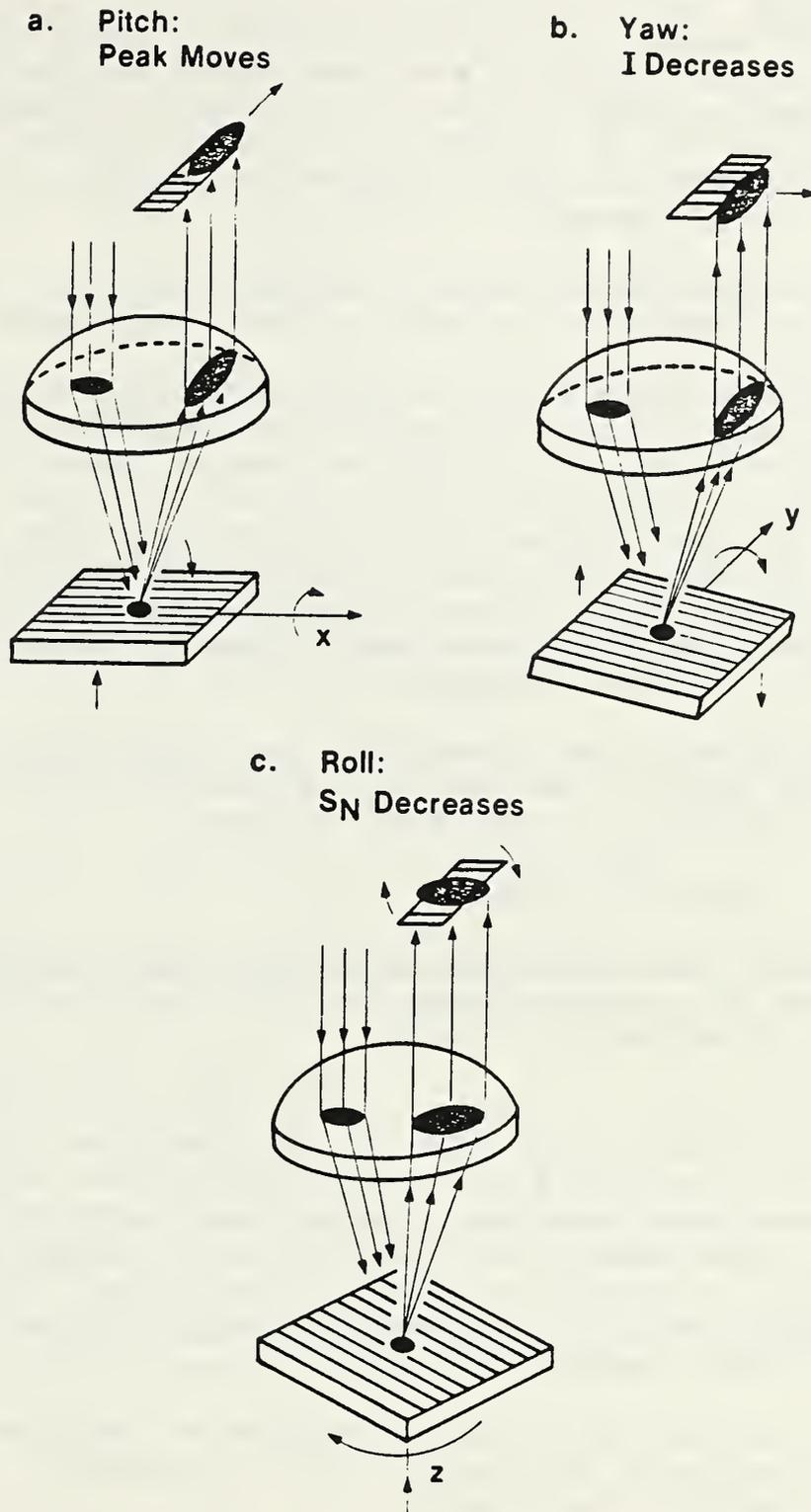
Figure 6. Details concerning optical alignment errors
