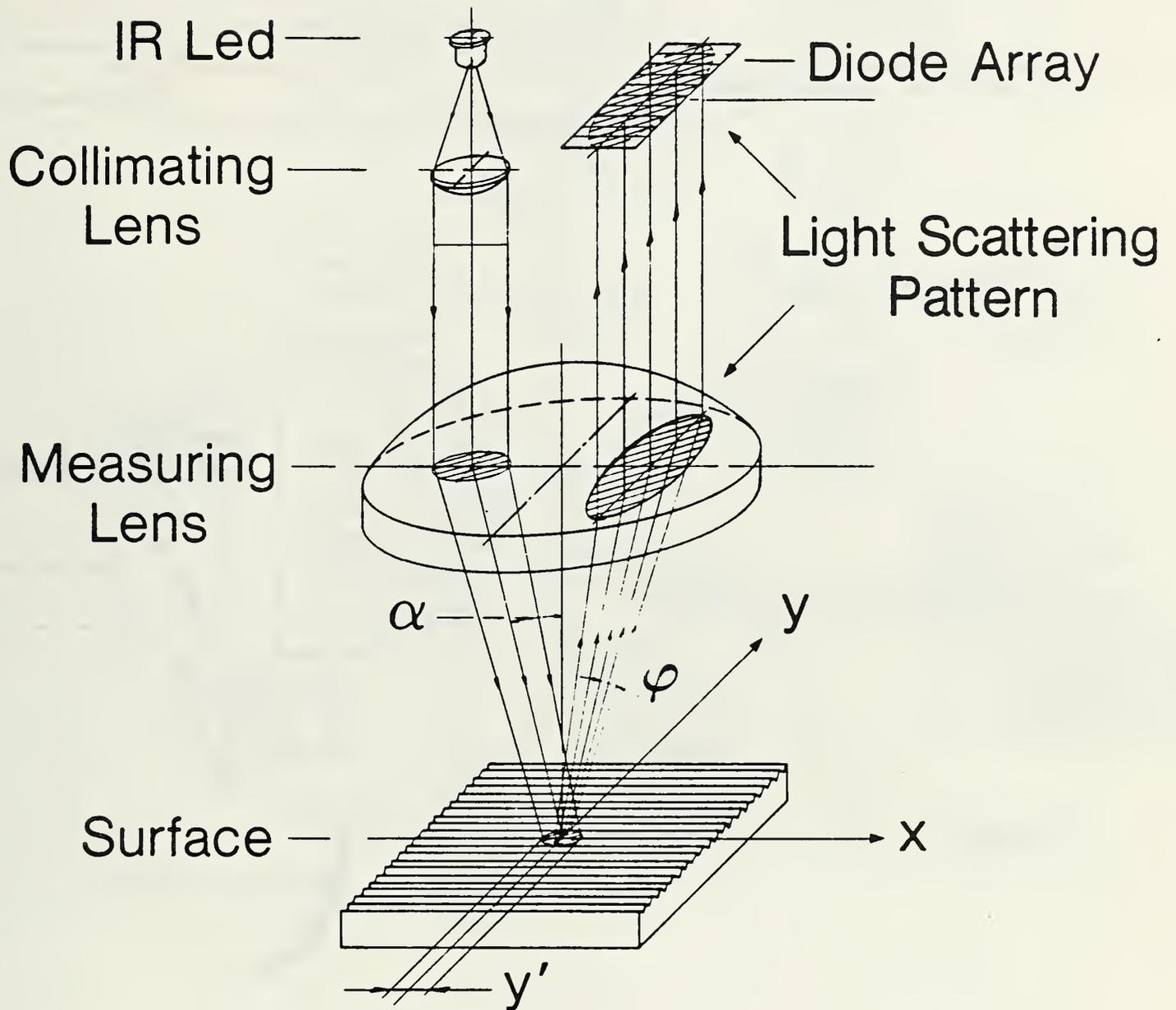
Figure 2. Schematic diagram of the optical system of the SRI
