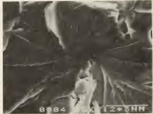
Figure 7. Cleavage fracture surface showing fine river pattern. A single cleavage facet is located at the center of the river pattern.
