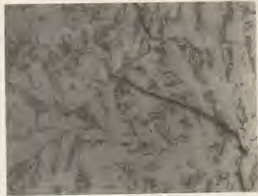
Figure 13. Cleavage microcracks which become arrested or deflected at the grain boundaries. (The micrograph was taken at a distance of 200  $\mu\text{m}$  to 300  $\mu\text{m}$  ahead of the fatigue crack tip.)
