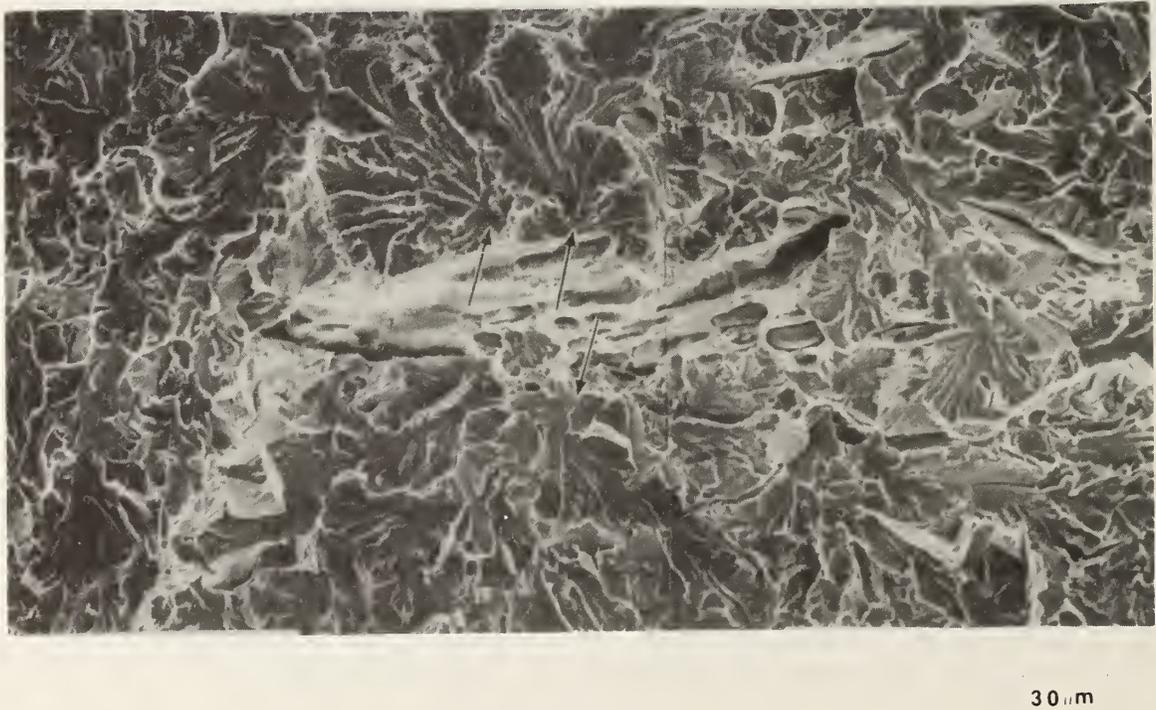
Figure 11b. Cluster of large inclusions in the center of the river pattern; a number of single cleavage initiation sites form the center of the fine pattern at the border of the cluster.
