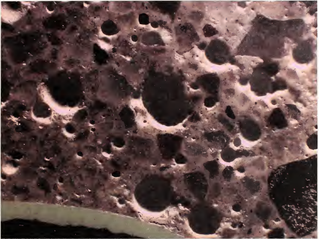
Figure 28. Snake River large core about -75 mm depth showing the paste bond to the epoxy-coated rebar and the entrained air void system.
