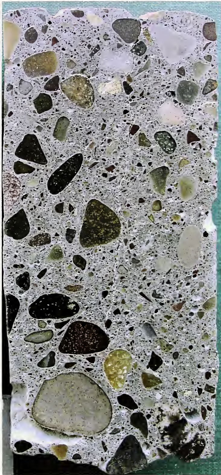
Figure 31. Snake River bridge core #4 (50 mm width) contains a full-core depth crack and some large entrapped air voids, mortar-rich regions and abundant entrained air.
