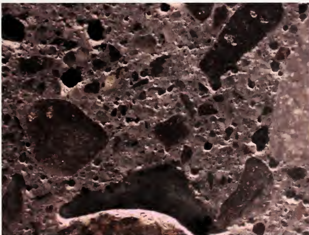
Figure 33. Snake River core #4 at (upper) 32 mm field width and (lower) 10 mm field width showing large entrapped air voids and high air content.
