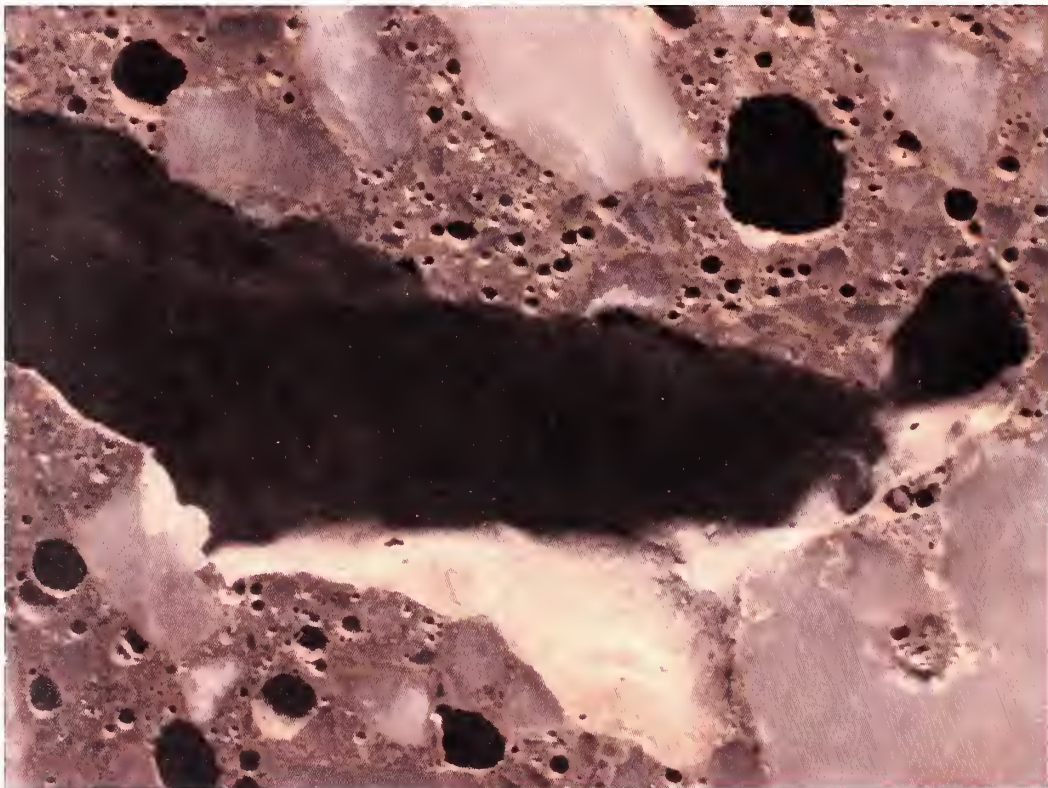
Figure 20. Darker, relatively air-free paste adjacent to the coarse aggregate is present in some cases, suggesting retempering (upper image, 10 mm field width) while large entrapped air voids (lower image) are common throughout the core.
