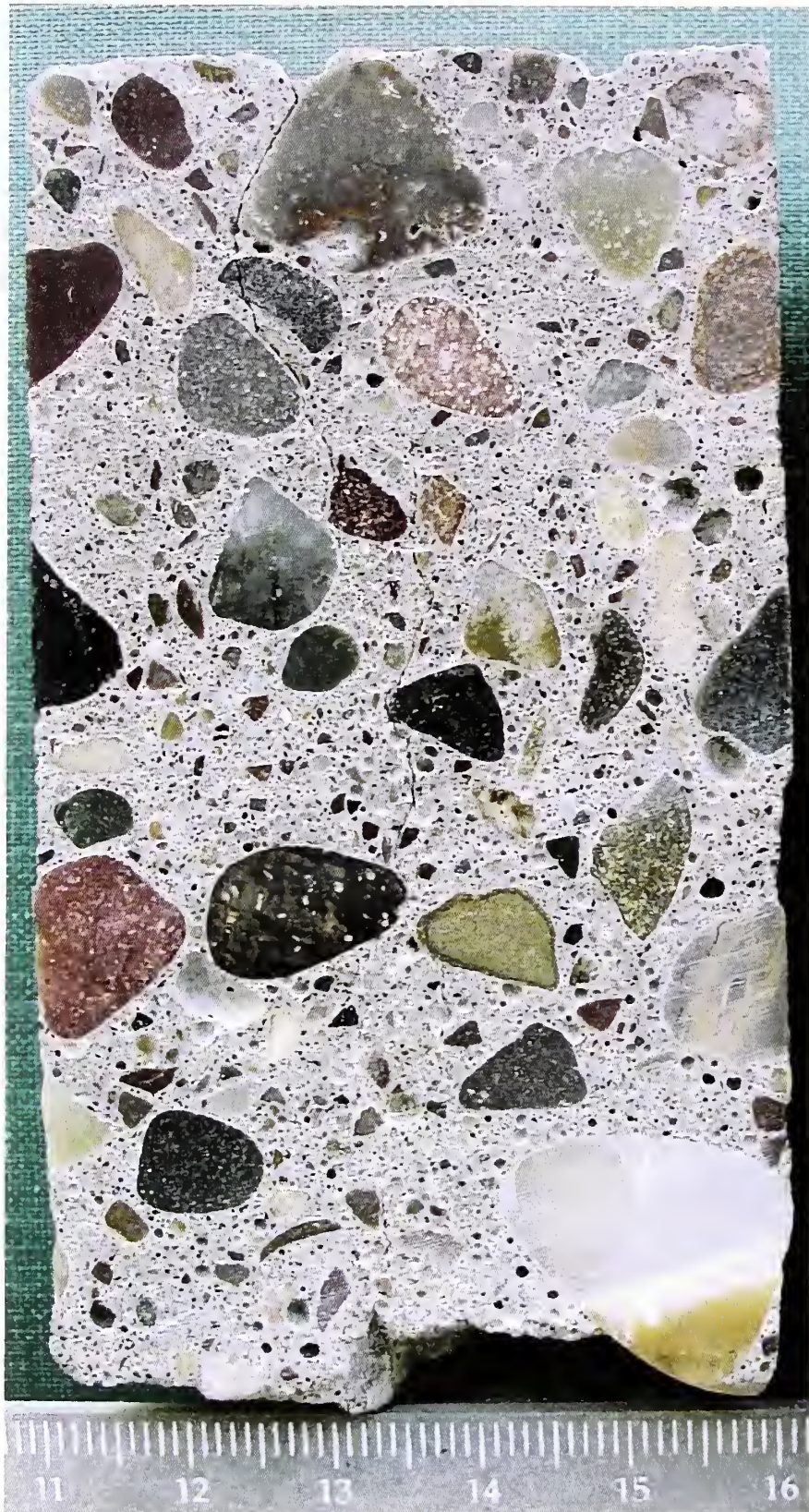
Figure 30. Snake River bridge core #3 showing a full-core depth crack, and high air content.
