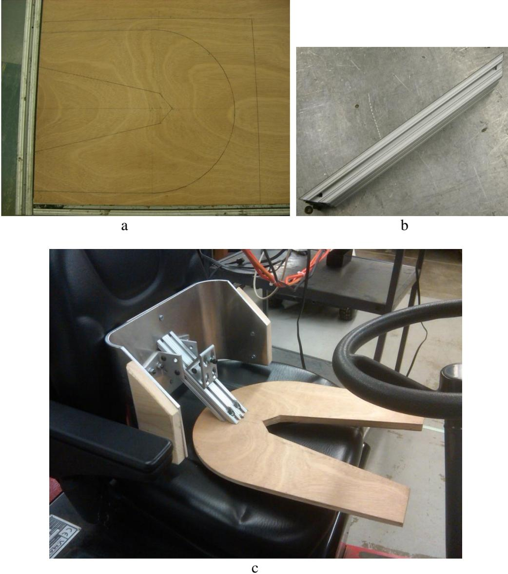
Figure 17. (a) SIP Apparatus: (a) base drawn on a piece of wood (b) joining bar for base to back, (c) fully assembled apparatus on a forklift seat.
