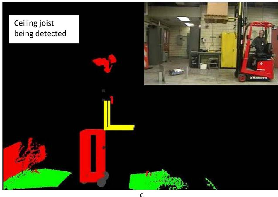
Figure 21. 3D imagers mounted on a forklift and integrated with simple operator alerts – (a) obstacle is behind the forklift and (b) the alert indicates the obstacle, (c) high lift obstacle detect sensor mounted to forks frame (upper right photo) capturing data of ceiling joists (lower left).
