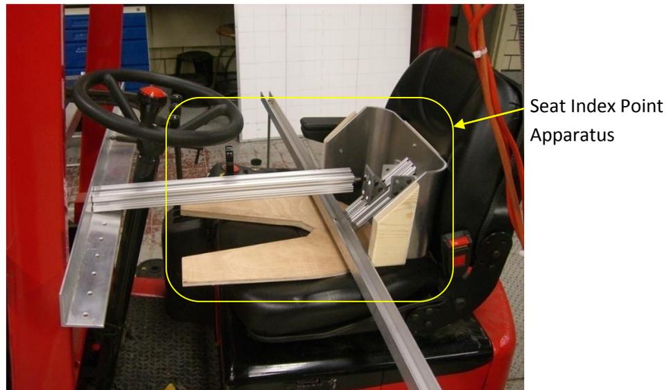
Figure 4. Seat Index Point Apparatus (a) as specified in ISO 5353 showing top (left drawing) and side (right drawing) views and (b) as-built by NIST ISD.
