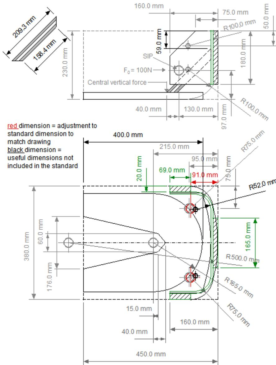
Figure 18. SIP Apparatus drawing showing standard drawing in gray and red, black and green modifications for NIST experiments.
