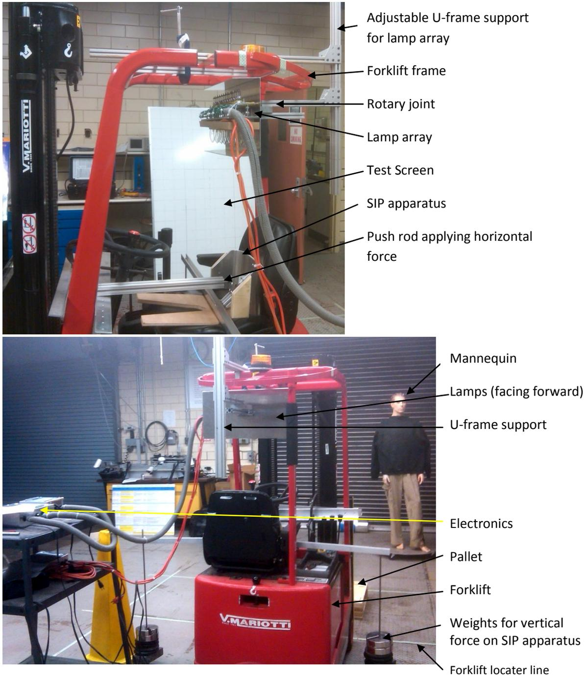
Figure 7 – Experimental setup showing all components.
