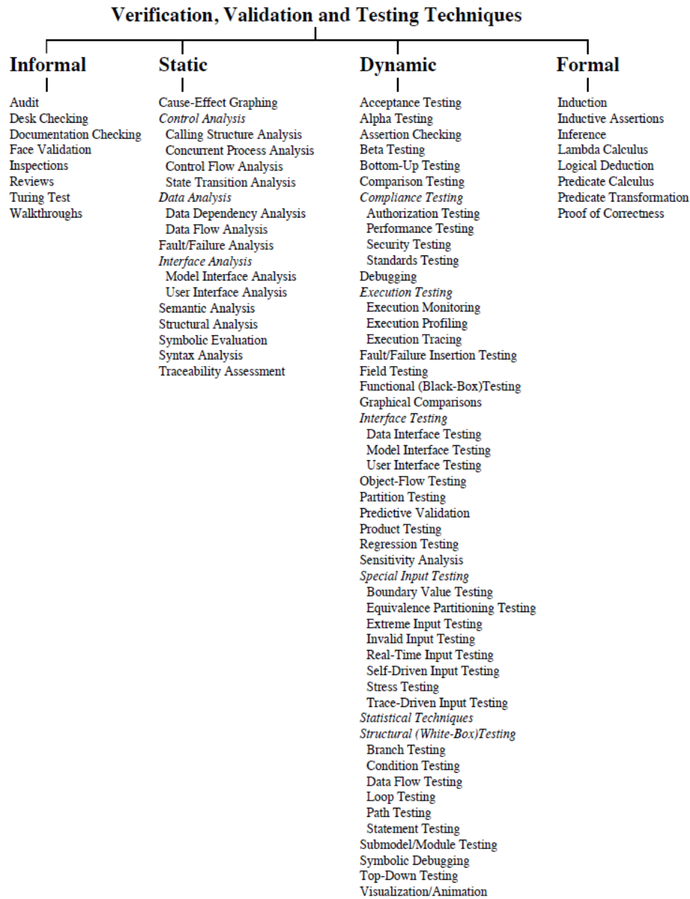
Figure 6: Taxonomy of Verification, Validation, and Testing Techniques (from [Balci 1998])
