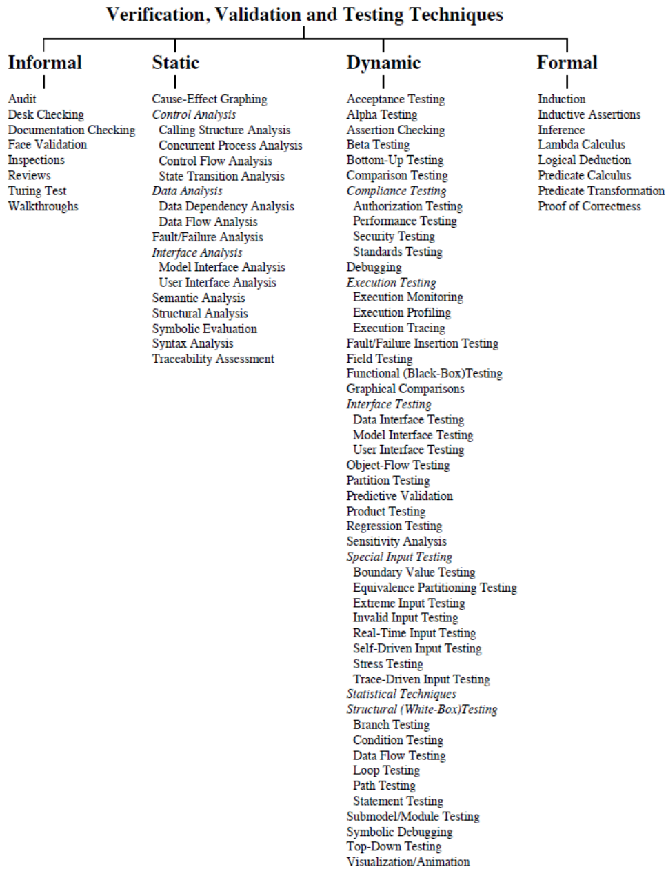
Figure 7: Taxonomy of Verification, Validation, and Testing Techniques (from [Balci 1998])
