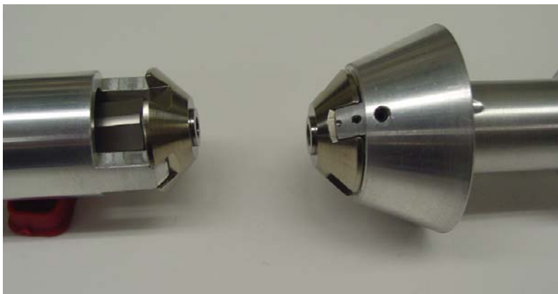
Figure 3c. Wrenches for attaching and removing mounting tables, shown with tables loaded on wrench
