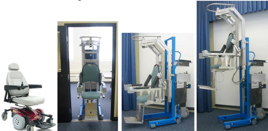
Figure 1: Typical powered chair (left) [courtesy Jazzy<sup>1</sup>] and the HLPR Chair 1 prototype (right three photos). HLPR Chair is shown in the mobility (center photos) and the lift (left-most) configurations. Note the unique shape of HLPR Chair as compared to typical powered chairs.
