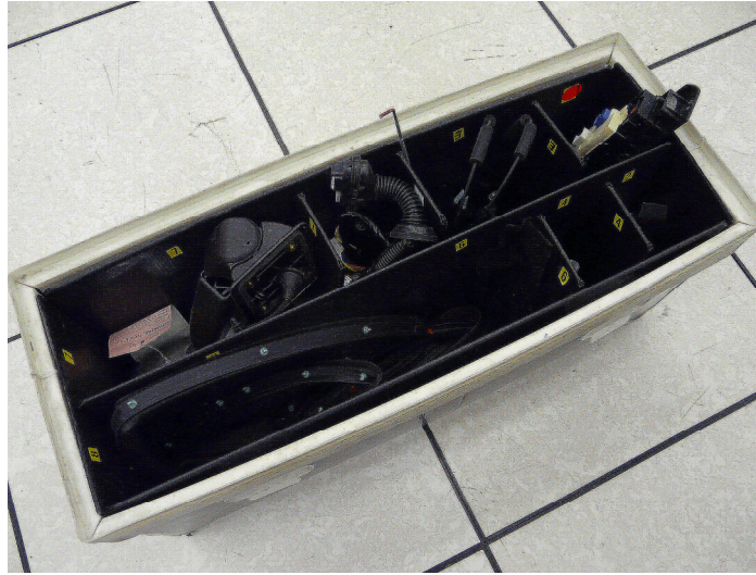
Figure 2. An example of filled kit with seven parts for a car door assembly task.
