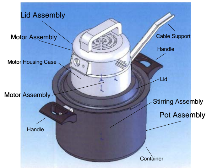
Figure 10: Automatic Pot Stirrer components [24]
