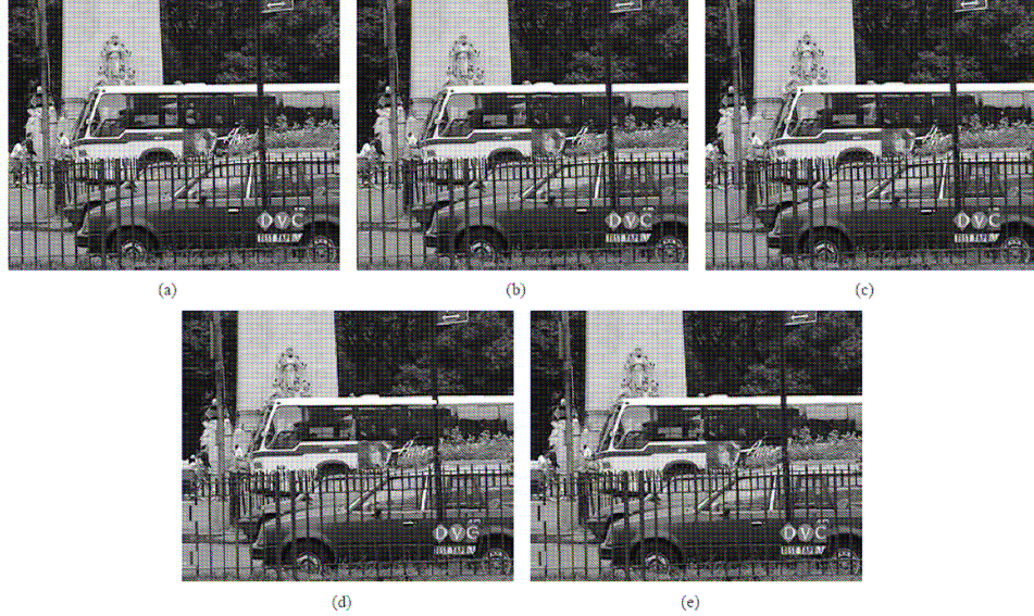
Fig. 6 Restored 34th frame of "Bus" CIF sequence when QP is 24. (a)error-free frame (37.93 dB); (b)MC frame (29.96 dB); (c)concealed with FC (16.57 dB); (d) concealed with PMVE (24.75 dB); (e)concealed with HMVE (26.14 dB). Gains over FC and PMVE are 9.57 dB and 1.39 dB respectively).
