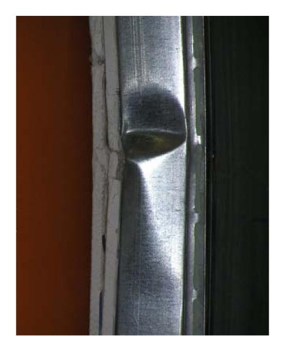
Figure 9 Close-up view of Local Buckling of C-H Stud – Specimen 3
