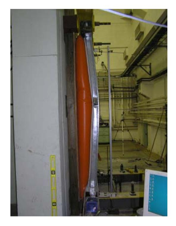
Figure 5 Post-test Photograph of Specimen 2 4 inch C-H Stud
