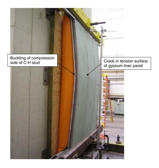
Figure 3 Post-test Photograph of Specimen 1 2-1/2 inch C-H Stud
