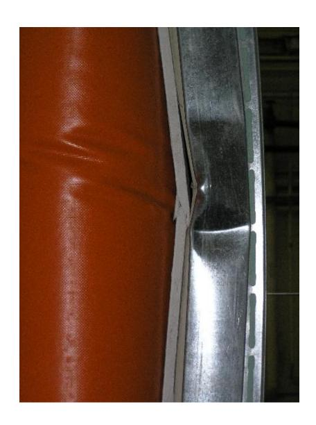
Figure 6 Close-up view of Local Buckling of C-H Stud - Specimen 2
