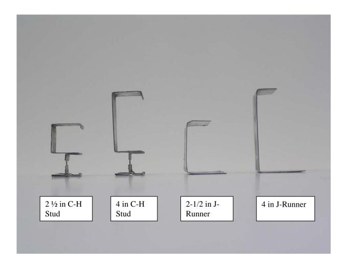
Figure 1 Cross Section of C-H Studs and J Runners
