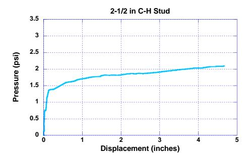
Figure 4 Air-bag pressure vs. panel center deflection plot of Specimen 1
