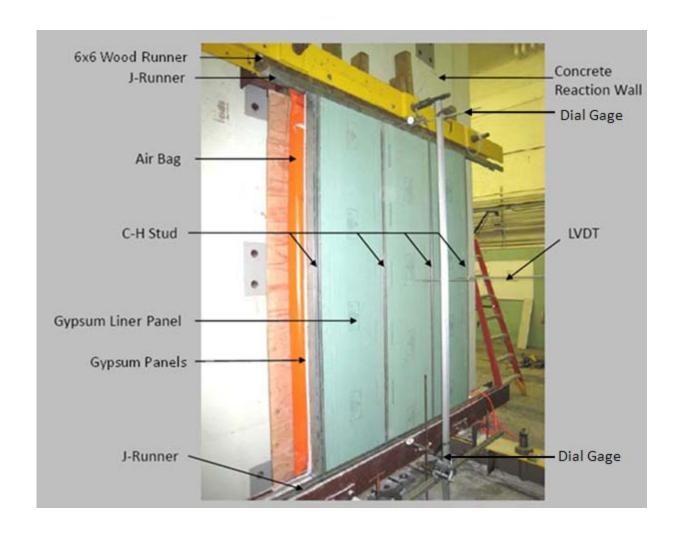
Figure 2 Test Setup
