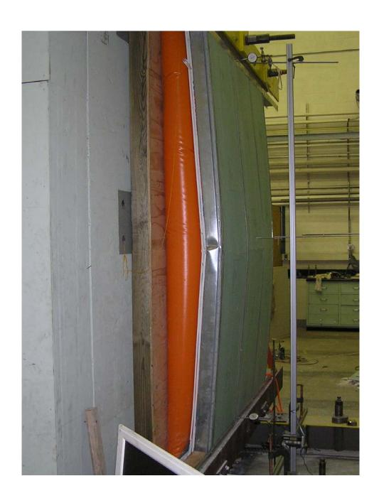
Figure 8 Post-test Photograph of Specimen 3 (4 inch C-H Stud)
