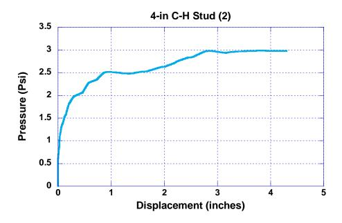
Figure 10 Air-bag pressure vs. panel center deflection plot of Specimen 3
