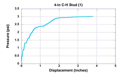
Figure 7 Air-bag pressure vs. panel center deflection plot of Specimen 2
