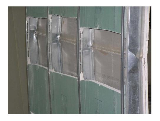
Figure 11 Development of local buckling in all four C-H studs - Specimen 3
