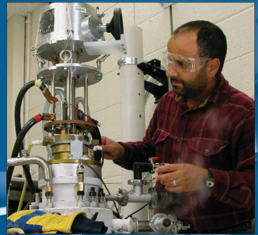
Figure 1. Unified apparatus for the measurement of superconductor critical-current density as a function of magnetic field, mechanical strain, and temperature.
