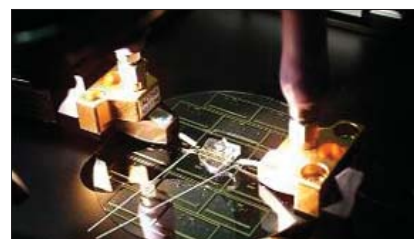
Figure 2. Integration of microwave elements with microfluidic systems for pinpoint temperature control and cycling (Shah et al., J. Micromech. Microeng. 2008; 17: 2224-2230).
