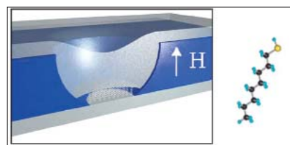
Figure 2: Schematics of a nanopore device with a monolayer of self-assembled molecules and the chemical structure of the octanethiol molecule. The arrow shows the direction of an applied magnetic field.
