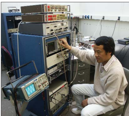
Figure 1. Setting up an automated system for determining the frequency dependence of fused-silica capacitors.
