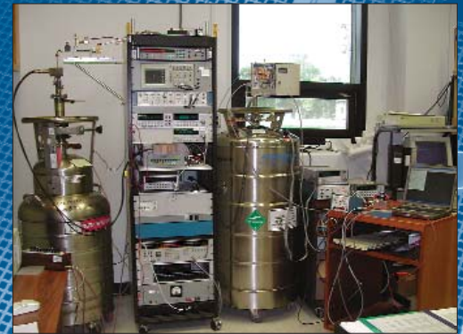
Figure 1. Set up the direct JVS comparison between the NRC JVS, Canada, and NIST compact JVS.
