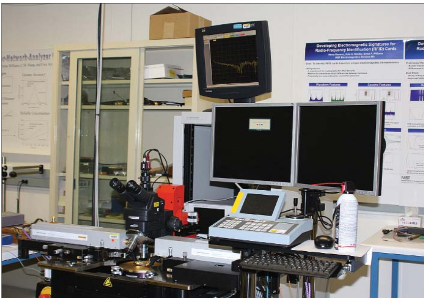
Figure 1. Probe station for making automated on-wafer device measurements.
