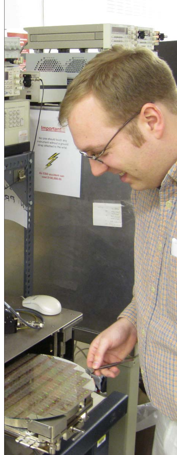
Figure 1. Loading 12" wafer containing state-of-the-art CMOS devices into a probe station in preparation of making high-speed measurements of transient changes in device characteristics due to temperature-bias stress.
