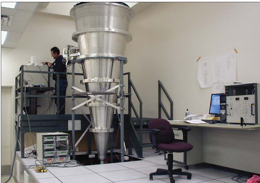
Figure 1. The co-conical field generation system developed by EEEL in preparation for testing.
