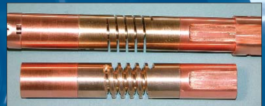
Figure 2. Two copper-alloy spring sample holders. Superconductor wires are soldered to the outer circumference of the springs. Torque applied to the spring puts the wires into tension or compression.
