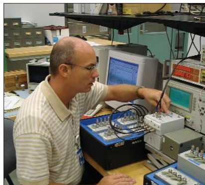
Figure 2. Performing a special test for a four-terminal-pair capacitance standard.
